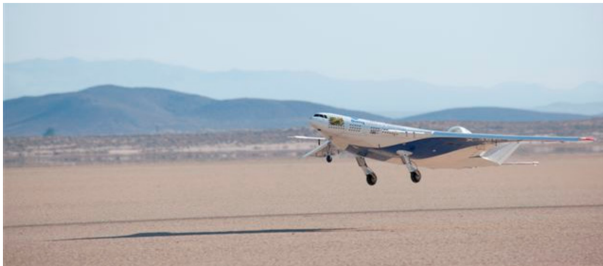
FIGURE 1.10 The NASA X-48C, which is a remotely piloted model of a hybrid wing body aircraft, takes flight for the first time. This aircraft is used for developing new fuel efficiency technologies. SOURCE: NASA/Tony Landis.
