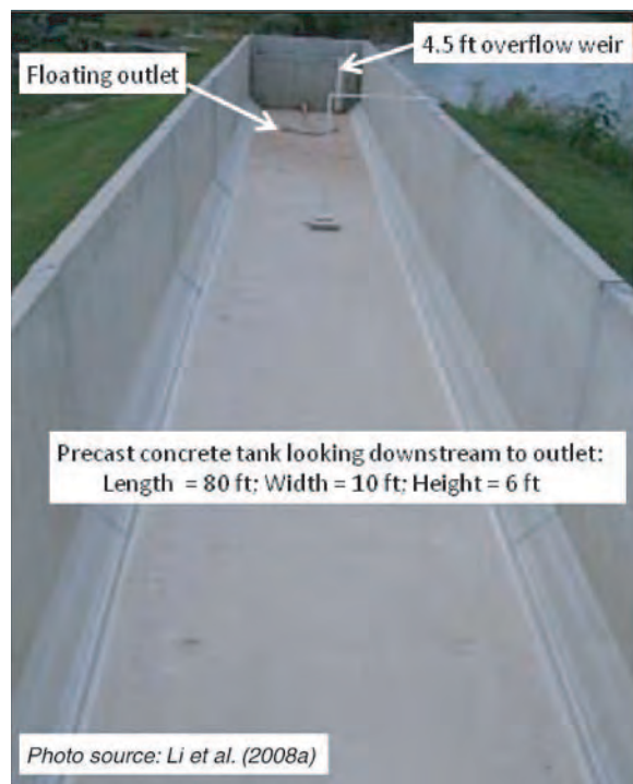
Figure 4.9. Non-proprietary precast concrete vault used in the Texas Transportation Institute to study sediment capture in prefabricated vaults.
