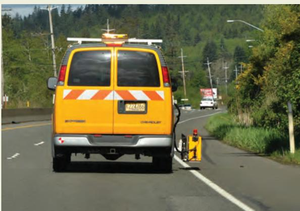
Washington State DOT works with Oregon DOT to rent an expensive, laser-equipped vehicle for collecting road stripe retroreflectivity data. According to the FHWA's Roadway Safety Data Partnership, levels of roadway data practice differ between states; collaborative programs can establish common approaches.
