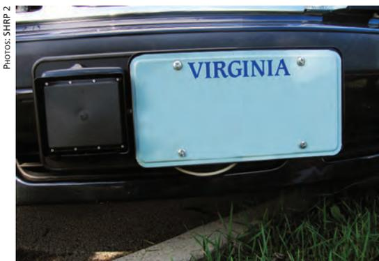
(Left:) A forward radar unit, mounted near the license plate, is among the data-gathering devices installed in participant vehicles.
