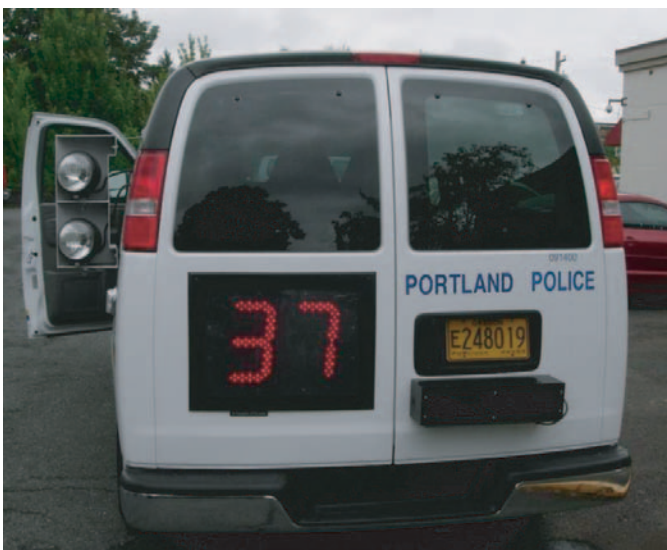
Figure H-3. Rear view of Portland's digital photo radar van.
