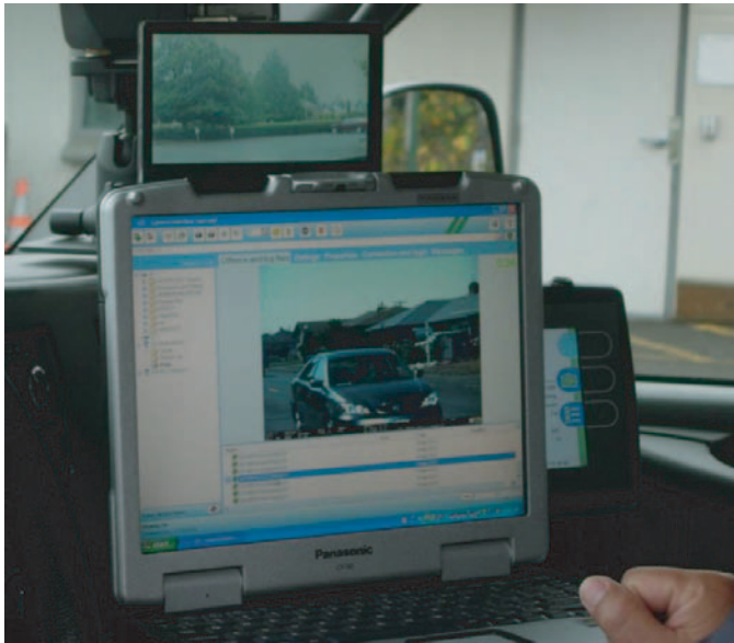
Figure H-4. Computer and camera monitor inside digital photo radar van.
