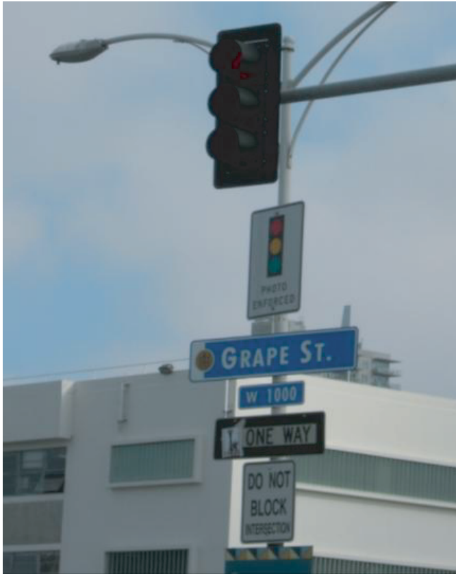
Figure H-21. Photo enforced signs are posted at every red light camera location. This one faces drivers on the approach to the intersection being enforced.
