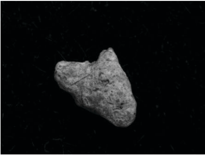
Figure 4-38. Crushed limestone (Brownwood, TX), #8-#16, magnification = 1.5.
