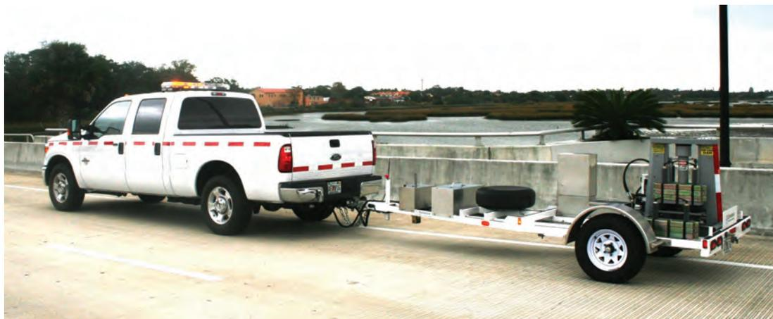
(Photo above:) A Florida DOT survey vehicle tows a falling weight deflectometer.
