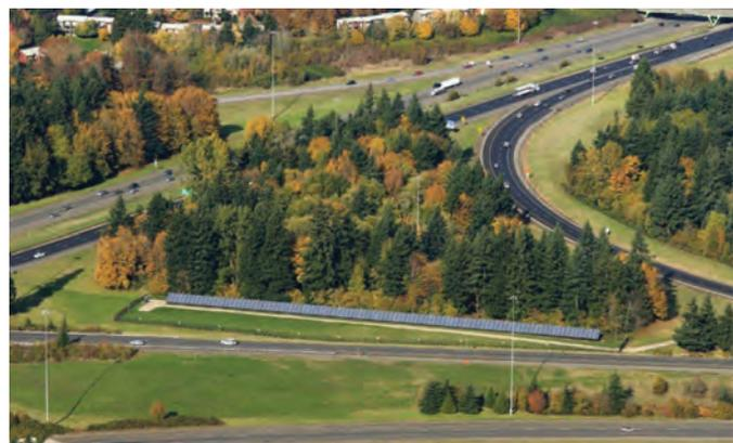
*Oregon DOT's first solar highway project, constructed in 2008, is a 104-kilowatt direct-current array located near a busy interchange south of Portland.*
