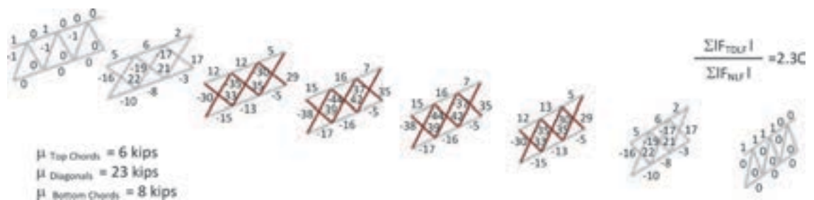
Figure 3-77. Bridge NISCR2 maximum amplitude of the component axial forces in each of the cross-frames under steel dead load, TDLF detailing of the cross-frames.
