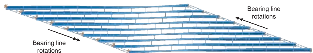
Figure 3-51. Bridge NISS54 “Configuration 3” deflected geometry under no-load due solely to the initial lack of fit associated with the TDLF detailing of the cross-frames (camber profiles based on 3D FEA vertical deflections).
