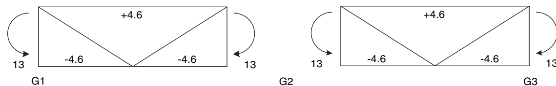
Figure 3-21. FHWA Test Bridge (EISCR1) unfactored (nominal) cross-frame dead load forces due to eccentric bracket loads (units: ft-kip moments, kip forces).
