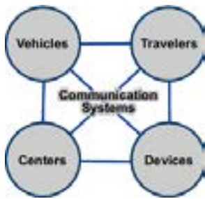
Figure 15. Interconnectivity between ITS system components.
