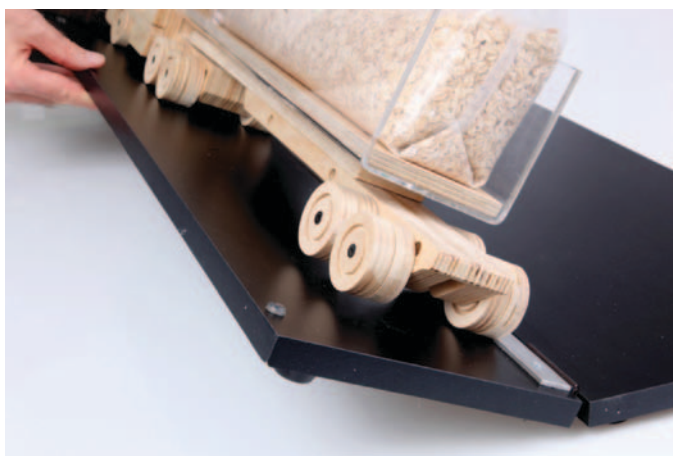
Figure 4. The trailer tips over at a lower angle with the oatmeal in the trailer than it does with an equal weight of sand.
