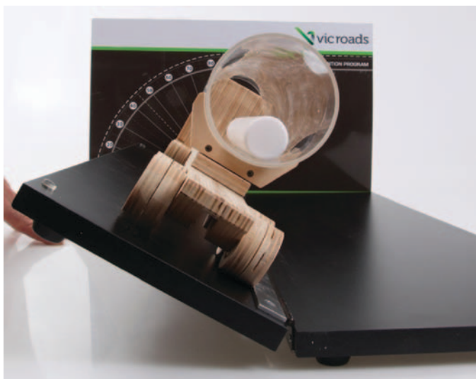
Figure 3. The rod in the cylinder simulates a liquid load in a tank. Note that the rod rolls toward the side even when the table is raised slowly.
