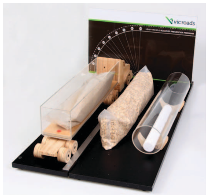
Figure 2. The VicRoads model truck on the tilt table; three loads are shown.
