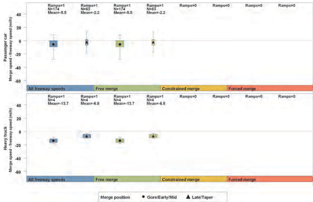
Figure 24. Merge speed differential by ramp type, merge type, vehicle type, and merge location (ramp type: loop; merge type: taper).
