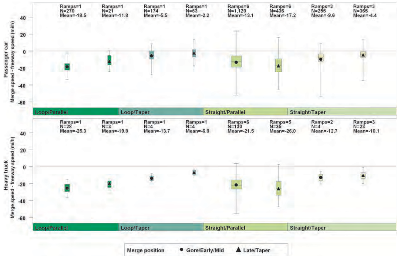
Figure 27. Merge speed differential by ramp type, merge type, vehicle type, and merge location (for free-merge conditions only).
