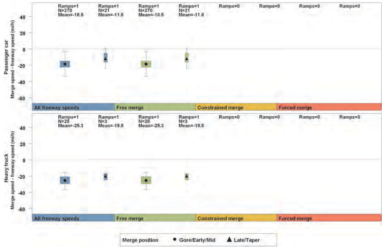
Figure 23. Merge speed differential by ramp type, merge type, vehicle type, and merge location (ramp type: loop; merge type: parallel).
