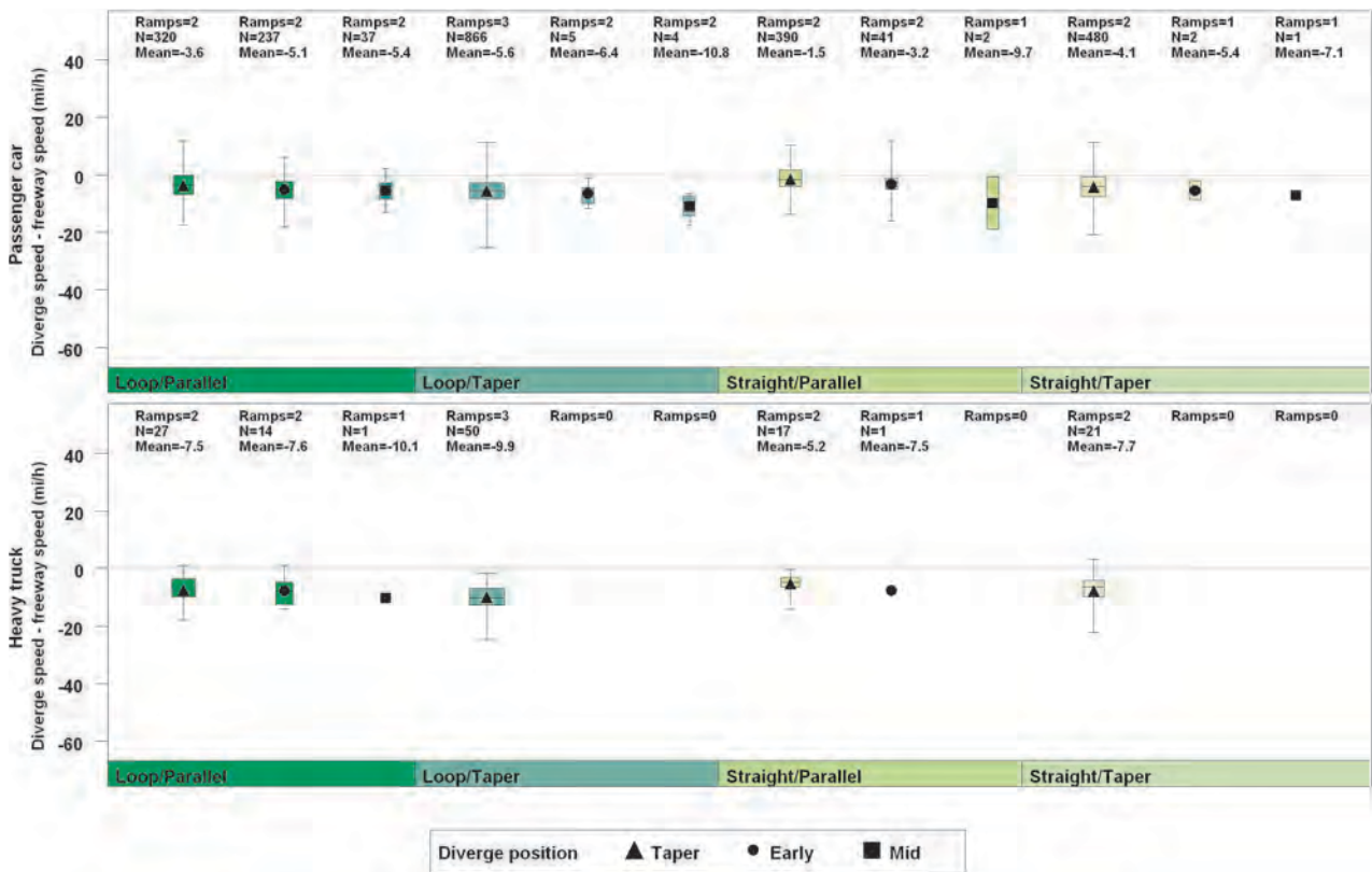
Figure 51. Diverge speed differential by ramp type, diverge type, vehicle type, and diverge location (for free-diverge conditions only).
