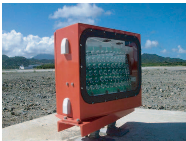
FIGURE 10 LED runway end identifier light.
