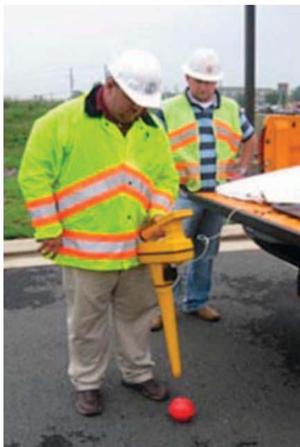
FIGURE 4 A marker ball RFID/Sonde being programmed prior to emplacement. (Photo courtesy of VDOT.)
