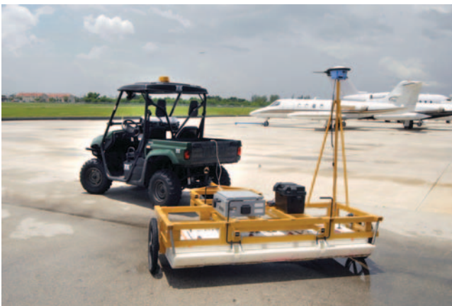
FIGURE 13 RTK GPS positioning on EMTC System at airport. (Photo courtesy of UIT.)
