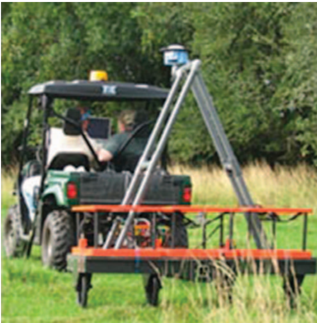
FIGURE 8 Multiple square antenna EMTC with integrated survey. (Photo courtesy of UIT.)
