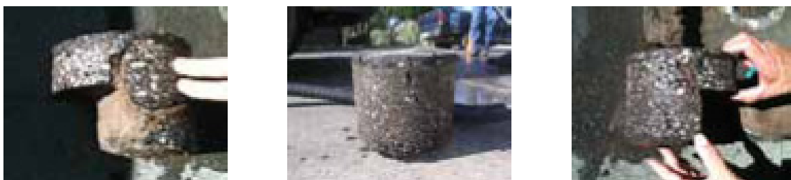
FIGURE 5 Cross-section view of cores taken from the Los Angeles County project.
