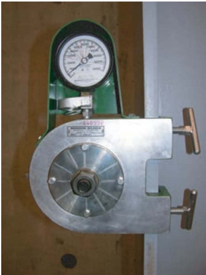
Figure 31. Skidmore-Wilhelm bolt load indicator.
