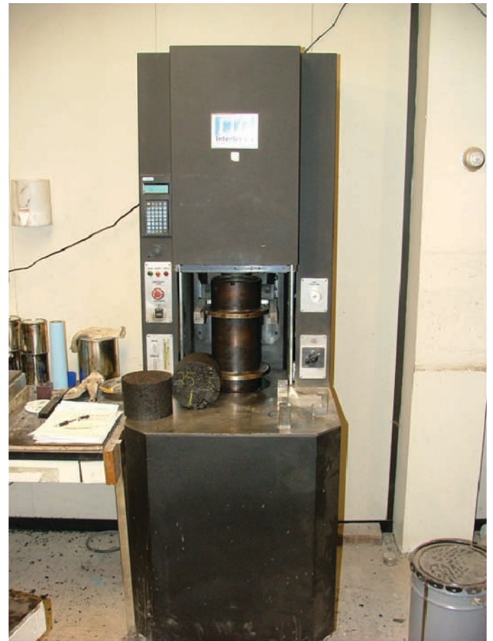
Figure 56. Interlaken gyratory compactor for compacting the HMA samples.
