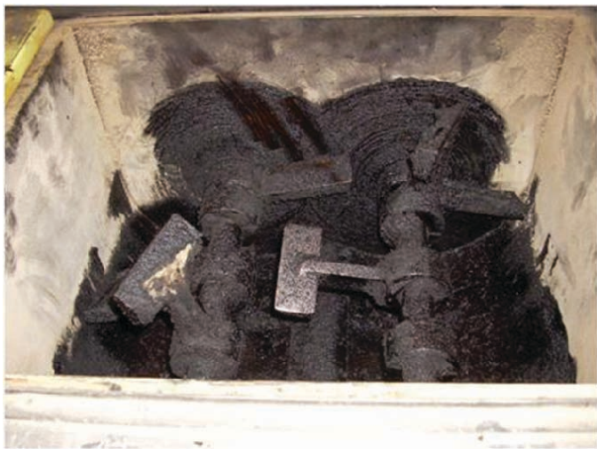
(b) Close-up of the paddles inside the pugmill mixer for mixing the HMA.
