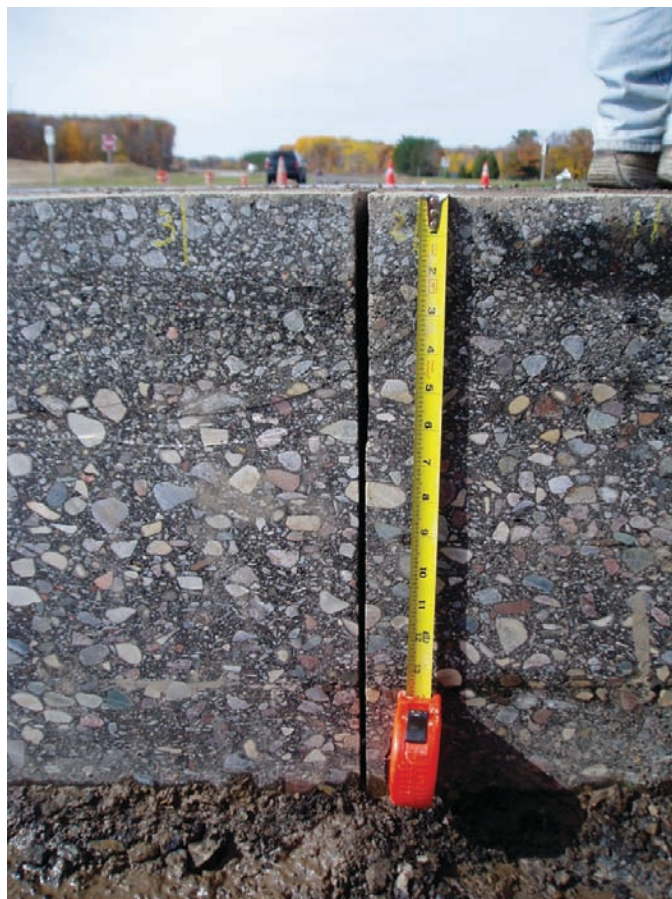
Figure 26. Forensic investigation of the Wisconsin SPS-1 project, test section 55-0116.
