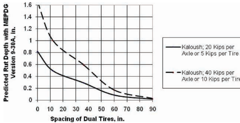
(b) Comparison of predicted rut depth using MEPDG Version 9-30A with a normal distribution of traffic loads.
