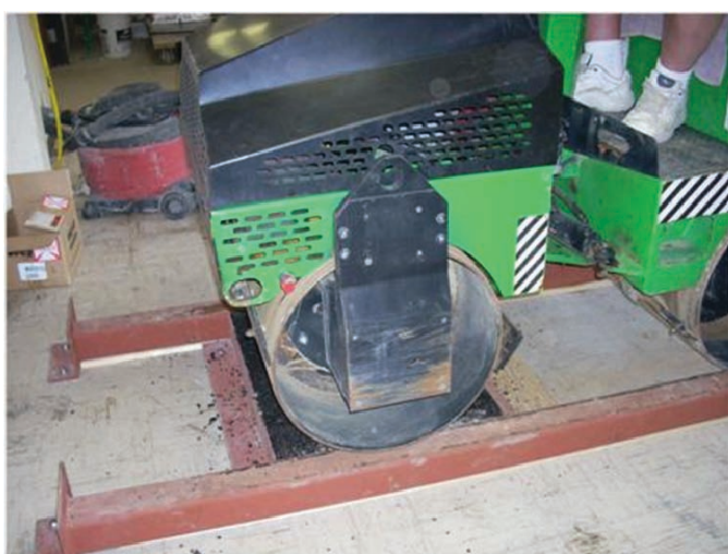
Figure 57. Self-propelled roller with a static steel drum weight of 3,000 lbs used to compact the shear test specimens.
