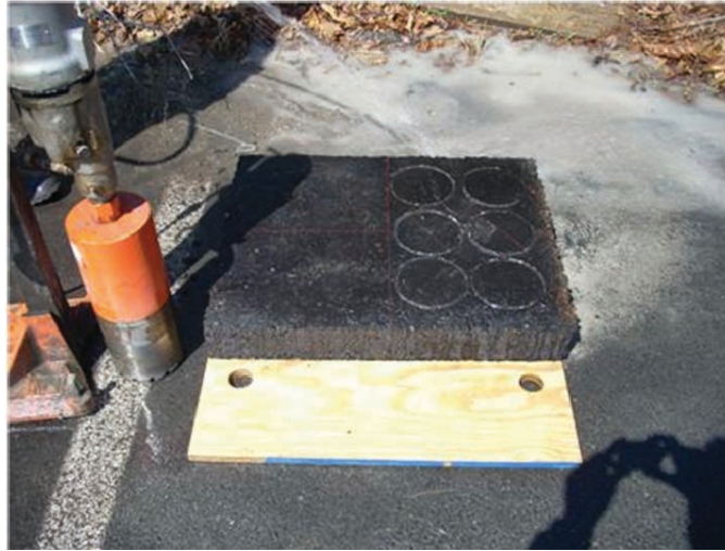
(a) Twelve cores being drilled from the HMA pad that was compacted with the rolling wheel compactor.
