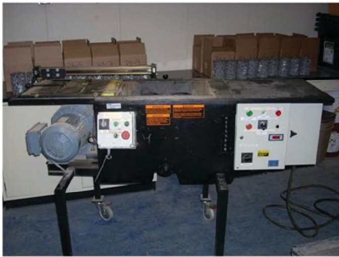
(a) Pugmill mixer or device used to mix and produce the HMA mixtures.
