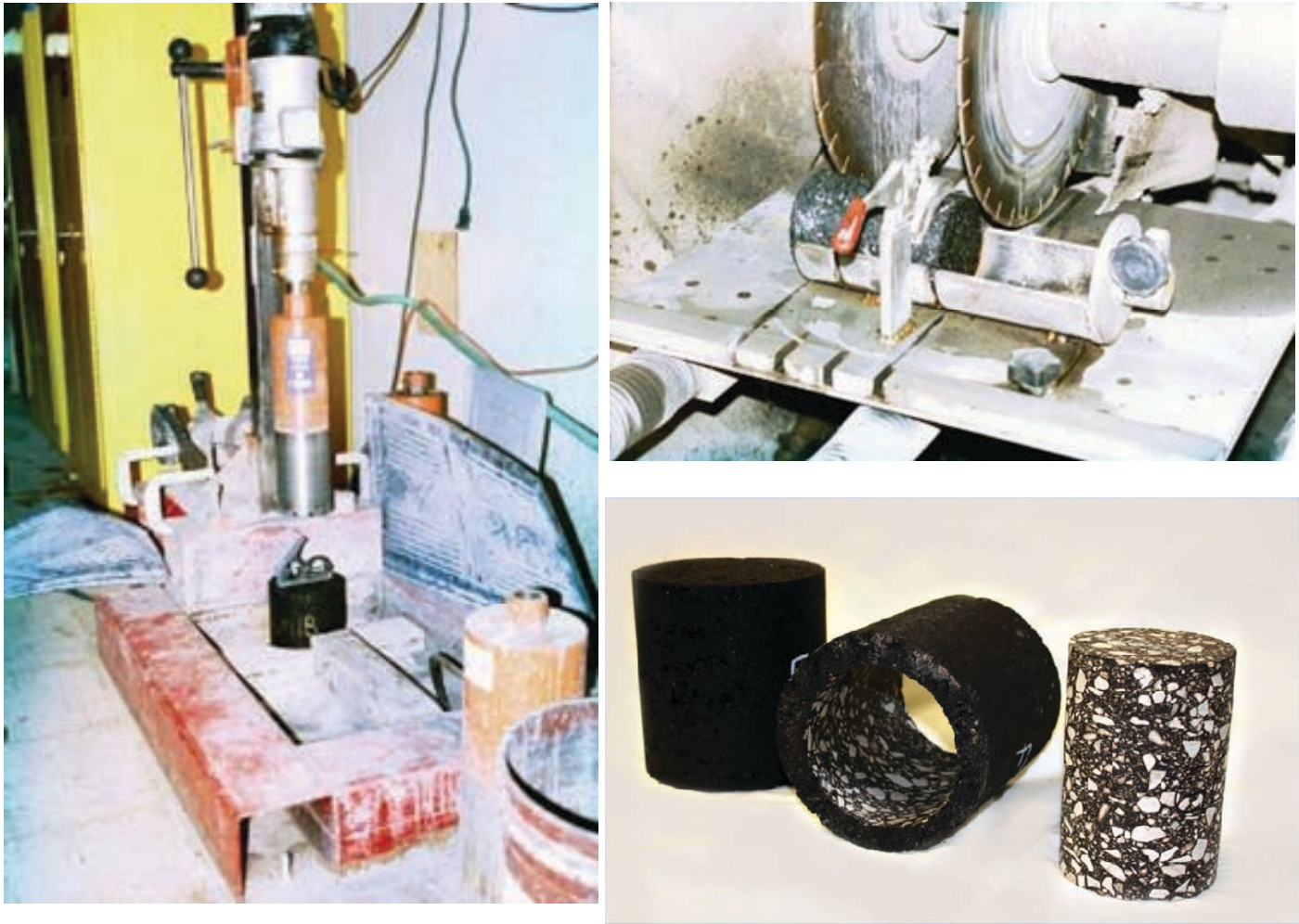
Figure 58. Coring equipment and operation for preparing the dynamic modulus and repeated-load triaxial test specimens.
