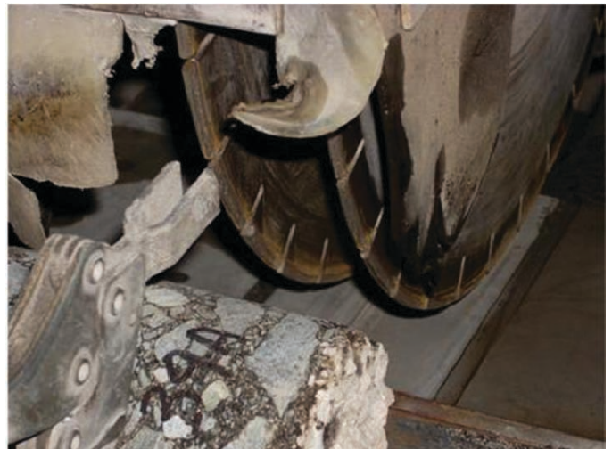
(b) and (c): A 50-mm-thick shear test specimen being sawed from the middle of the full depth core using a double-bladed saw to ensure that the ends were parallel.
