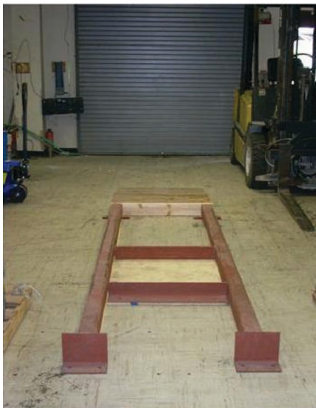
Figure 54. Fabricated rolling wheel mold used to compact HMA for the repeated-load constant-height shear test and the HMA pad from the rolling operation.
