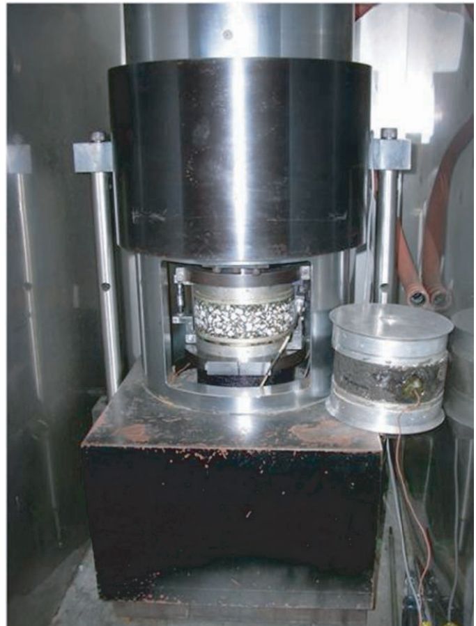
Figure 62. Test specimen setup for the repeated-load constant-height shear plastic deformation test.
