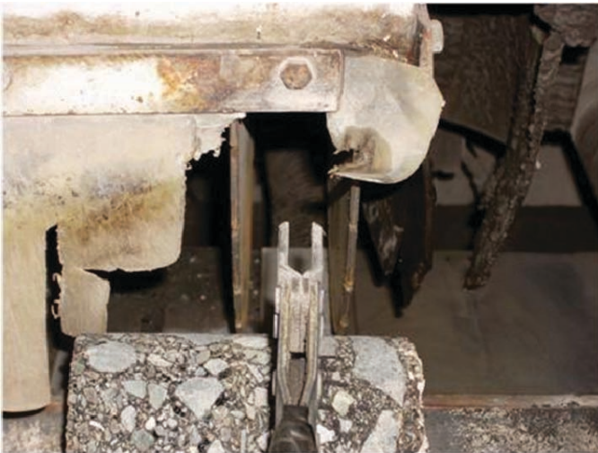
(b) and (c): A 50-mm-thick shear test specimen being sawed from the middle of the full depth core using a double-bladed saw to ensure that the ends were parallel.
