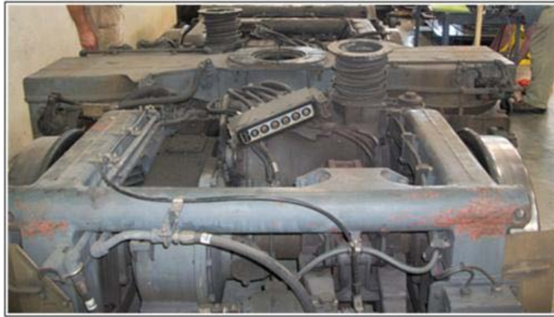
Figure 6. Hammer Test and SLRV Motor Truck
