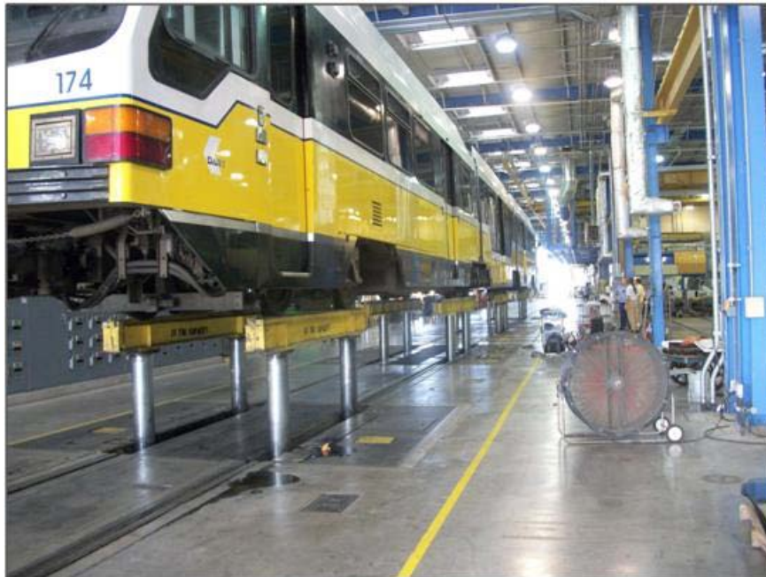
Figure 10. SLRV on Vertical Lift
