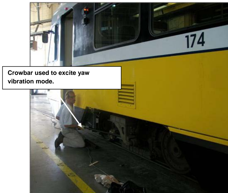
Figure 5. Using a Crowbar to Excite Carbody Yaw Vibration Mode
