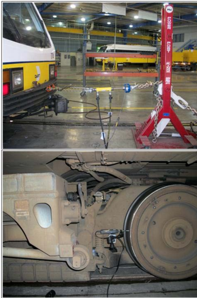
Figure 8. Setup of Longitudinal Pull Test
