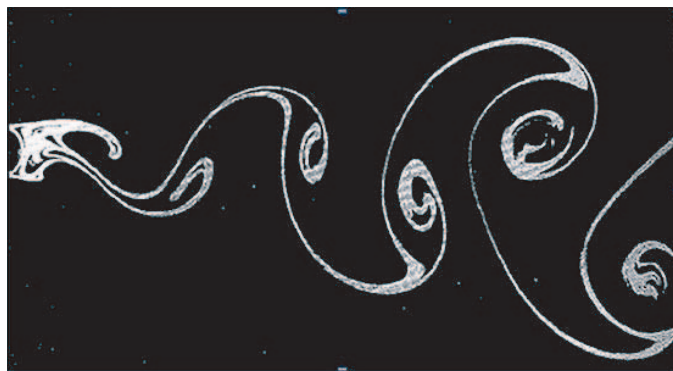
Figure 2.9. Picture of von Karman vortex street (Anderson, 2007).
