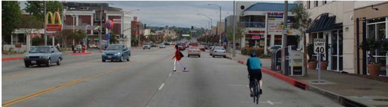
Existing conditions show a street designed for cars only, with a 40 MPH speed limit, a pedestrian attempting to cross without any break in traffic, and a cyclist traveling without benefit of a marked bicycle lane.
