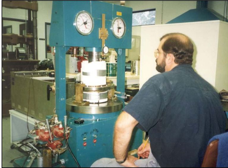
Figure 27 Modified Texas Six-Inch Gyratory Compactor at the Asphalt Institute. Note pressure gauges at top of machine, spring 1991
