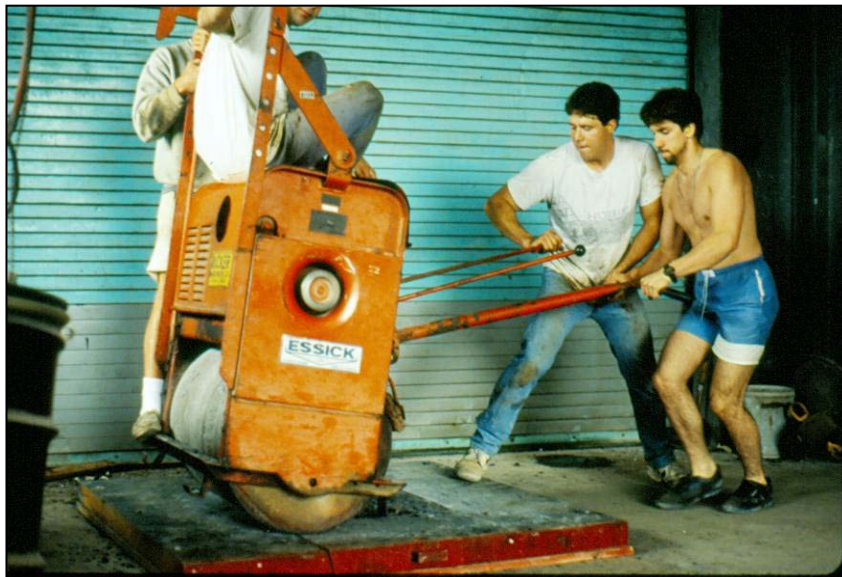
Figure 35 Students Compacting a Specimen by Rolling Wheel at University of California Berkeley, April 1991 (All persons are unidentified)
