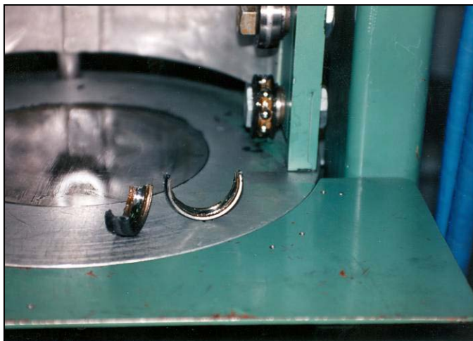
Figure 31 Bearing problems on first prototype Superpave gyratory compactor, Tomah, Wisconsin, July 8, 1992
