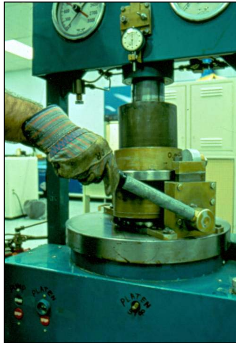
Figure 29 Angle is applied by rotating the handle and raising the side of the mold. Handle is removed before rotation (gyrations) start, spring 1991
