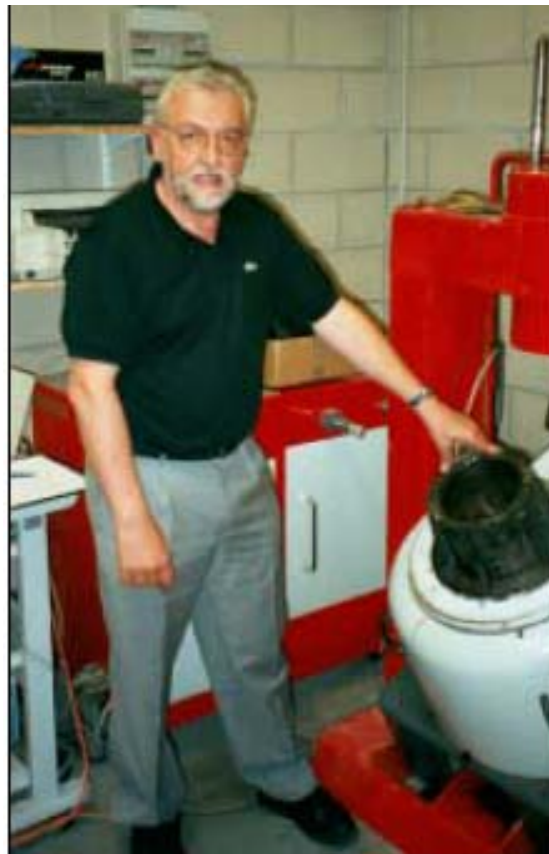
Figure 26 Francis Moutier with Second Generation LCPC Gyratory Compactor, circa 1998
