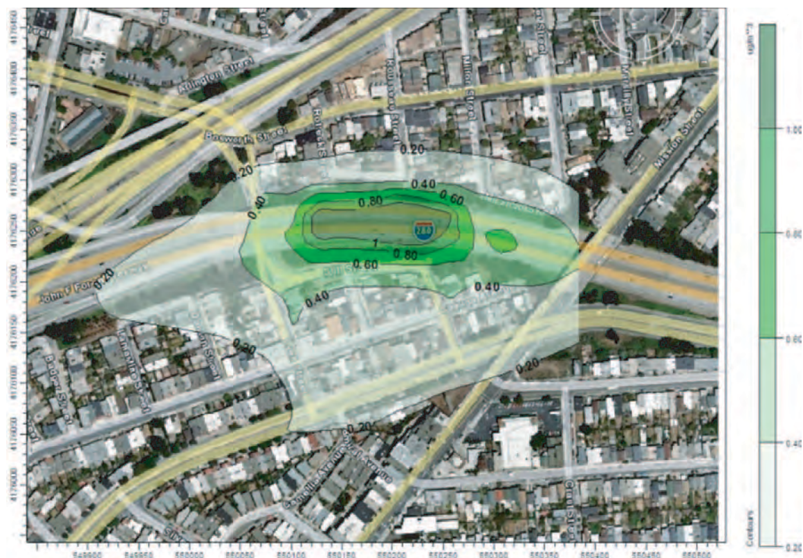
Figure 3-46. San Francisco's Public Health Department prepared a retroactive health impact assessment of traffic in Excelsior's Still/Lyell Freeway Channel. Highest-day cumulative exposure maps for PM 2.5 particulates were modeled and mapped to show freeway traffic, informal diesel truck routes, diesel bus routes, as well as neighborhood traffic volumes. The analyses assess and communicate additional public health risks associated with neighborhood traffic volumes.
