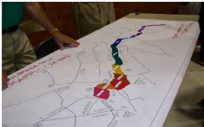
Figures 3-22 and 3-23. Visualizations used at public meetings involving comparisons of alternatives and different concepts for a specific location (top) and use of different colors and widths of lines to indicate size of traffic volumes (bottom).
