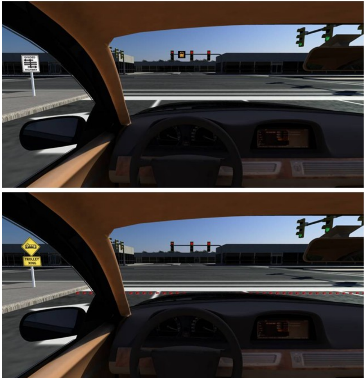
Figure 13. Cross-Street Scenarios with Various Traffic Signal Displays and Two Different Types of Active Traffic Control Devices (W10-7 Sign and In-pavement Lights)
