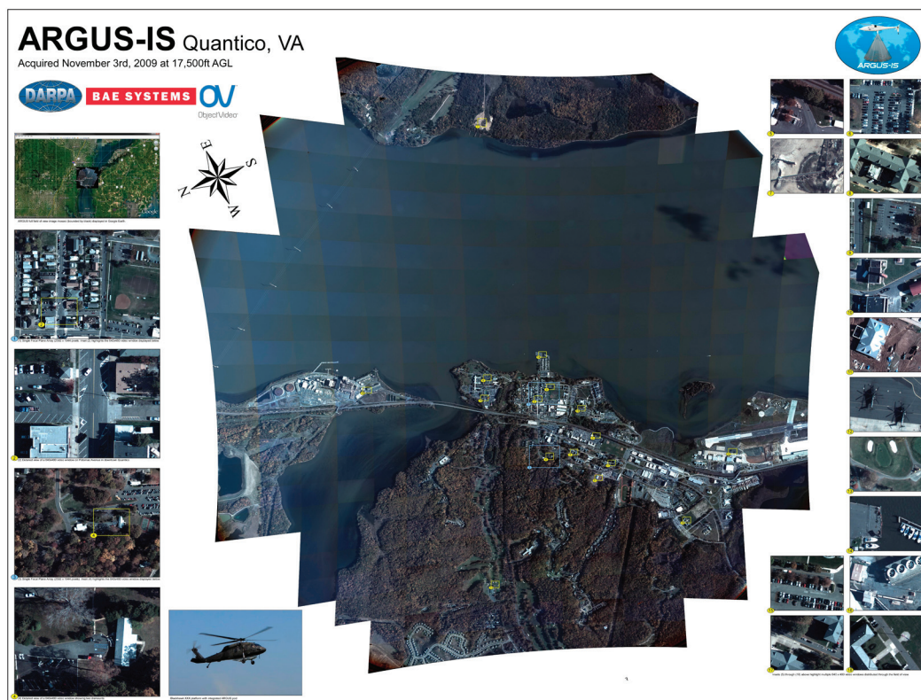
FIGURE 4.2 A sample of the ARGUS-IS imagery. The system was mounted under a YEH-60B helicopter flying at 17,500 feet over Quantico, Va. The Argus-IS images an area more than 4 km wide. The ARGUS system uses a large number of inexpensive cell phone cameras to create a whole new imaging modality with a huge format. SOURCE: Image available from DARPA Information Innovation Office, Autonomous Real-time Ground Ubiquitous Surveillance-Imaging System (ARGUS-IS), at http://www.darpa.mil/Our_Work/I20/Programs/Autonomous_Real-time_Ground_Ubiquitous_Surveillance-Imaging_System_%28ARGUS-IS%29.aspx .
