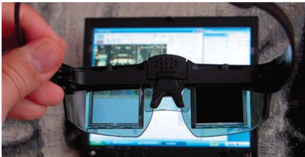
FIGURE C.20 Shutter glasses blocking left image from entering right eye. Image courtesy of E. Svedberg.
