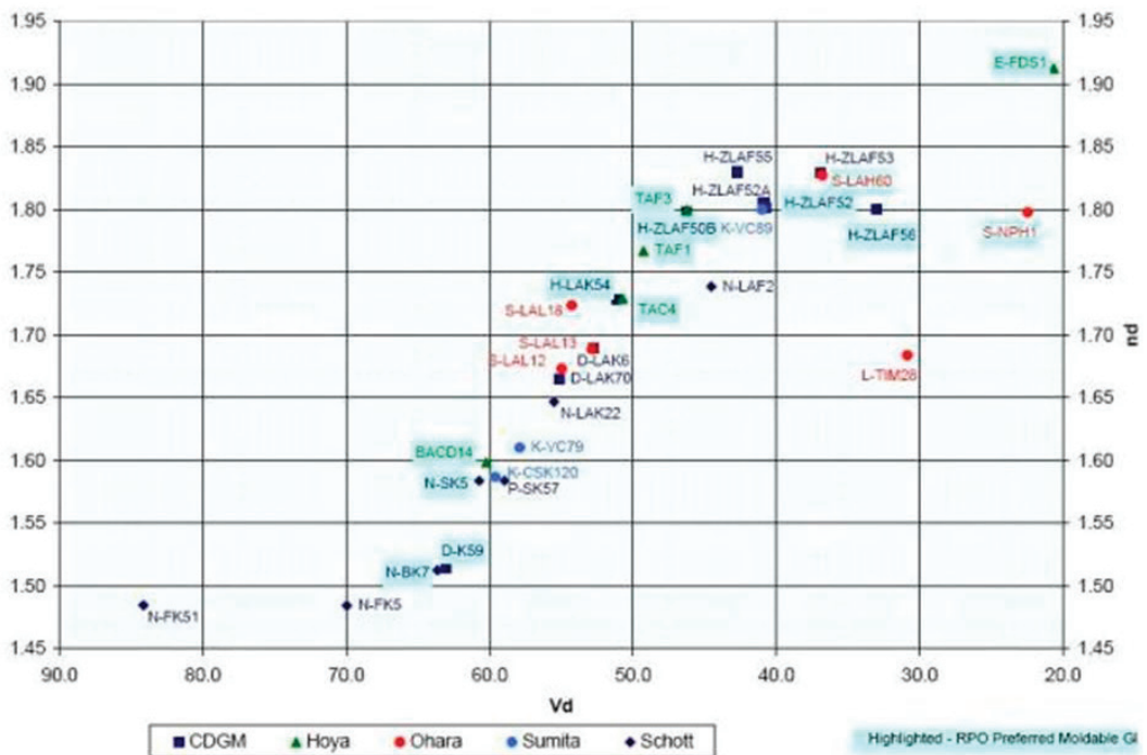
FIGURE C.11 Moldable glasses types available from Rochester Precision Optics. SOURCE: Courtesy of Rochester Precision Optics.
