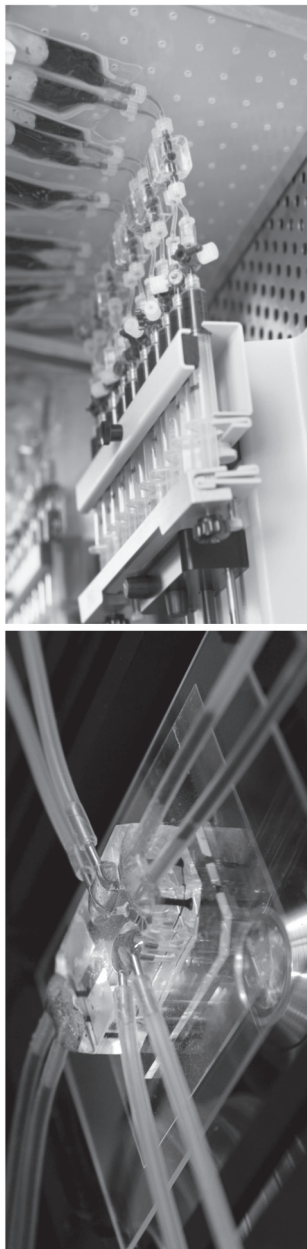
FIGURE 2 Examples of microfluidics (left, printed with permission from the Wyss Institute) and mesofluidics (right, KIYATEC Inc.) “layered complexity” in vitro systems. Both are perfusion based and incorporate 3D microenvironments and coculture interactions, but they differ in scale, manufacturing techniques, potential applications for cell-scaffold constructs, cost, and throughput.
