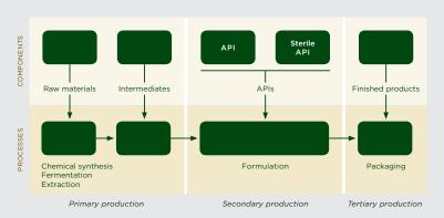
FIGURE 4-1 Schematic block diagram of a pharmaceutical manufacturing process. NOTE: API = active pharmaceutical ingredient. SOURCES: Adapted from Kaplan and Liang, 2005; Wilson et al., 2012.
