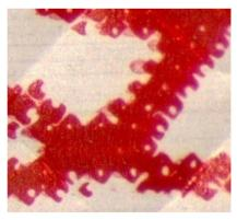
FIGURE 6-2 The printing on a fake Cialis blister pack is less crisp at 32× magnification. SOURCE: Lim, 2012.
