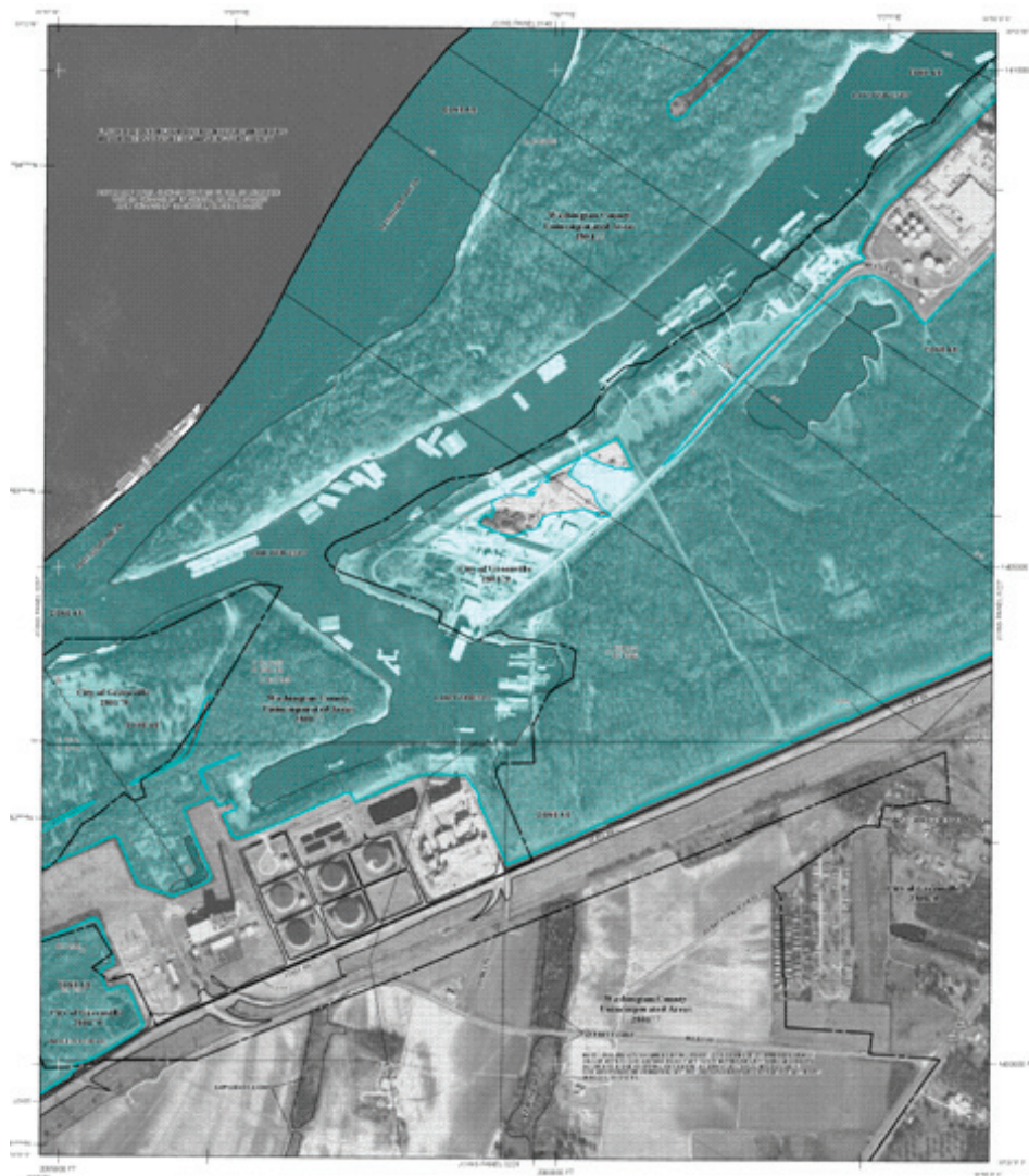
FIGURE 7-2 A Flood Insurance Rate Map for a section of Greenville, Mississippi, along the Mississippi River. The blue areas are within the SFHA (Zone AE) and the gray area (Shaded Zone X) represents areas behind accredited levees. SOURCE: FEMA Map Service Center. Available at http://map1.msc.fema.gov/idms/IntraView.cgi?KEY=93429510&IFIT=1
