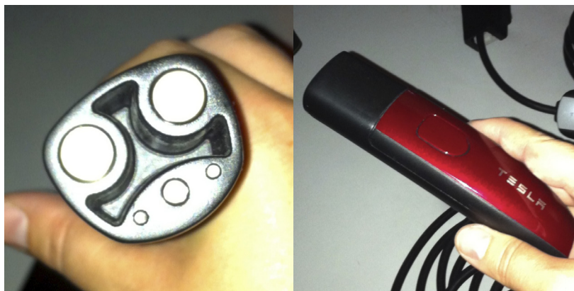
FIGURE D-4 The Tesla proprietary plug for DC fast charging is used for all Tesla DC fast chargers (Superchargers) now available in the United States. It is available only on the Tesla Model S. SOURCE: Gordon-Bloomfield (2011). Photo by Nikki Gordon-Bloomfield.
