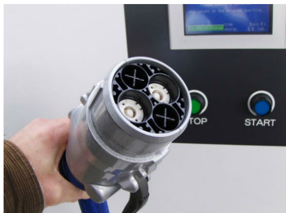
FIGURE D-2 The CHAdeMO plug for DC fast charging is used for most DC fast chargers in the United States, Europe, and Japan and is available on most battery electric vehicles that can accept DC fast charging. SOURCE: Brissette (2013).
