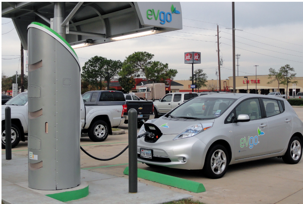
FIGURE 3-3 DC fast charging a Nissan Leaf. DC fast charging is able to charge a Nissan Leaf battery to 80 percent capacity in less than 30 min. The charge would typically allow a 2013 Leaf to travel about 64 miles. SOURCE: Copyright 2010 by the evgo Network; licensed under Creative Commons 2.0 (CC-BY-2.0).
