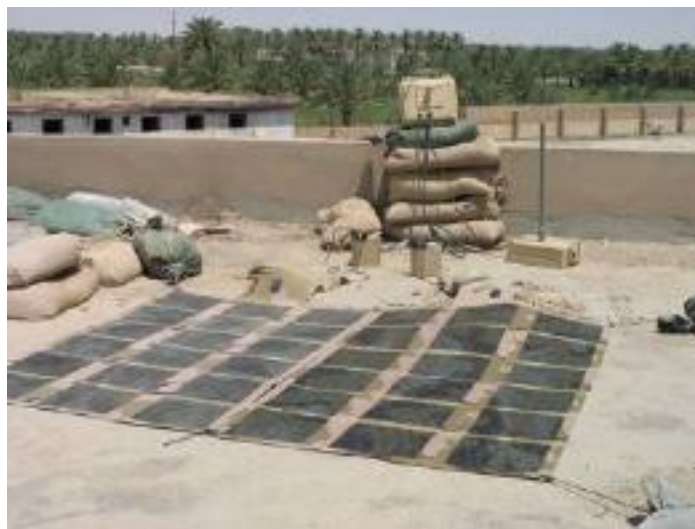
FIGURE I-2. Deployable portable solar array. SOURCE: Deanna Tyler and George Au, Army Power Division, “Assessment of the Army’s Need for Portable Energy,” presented at the DARPA Limits on Thermodynamic Storage (LOTS) of Energy Proposers’ Day Workshop, December 4, 2009.
