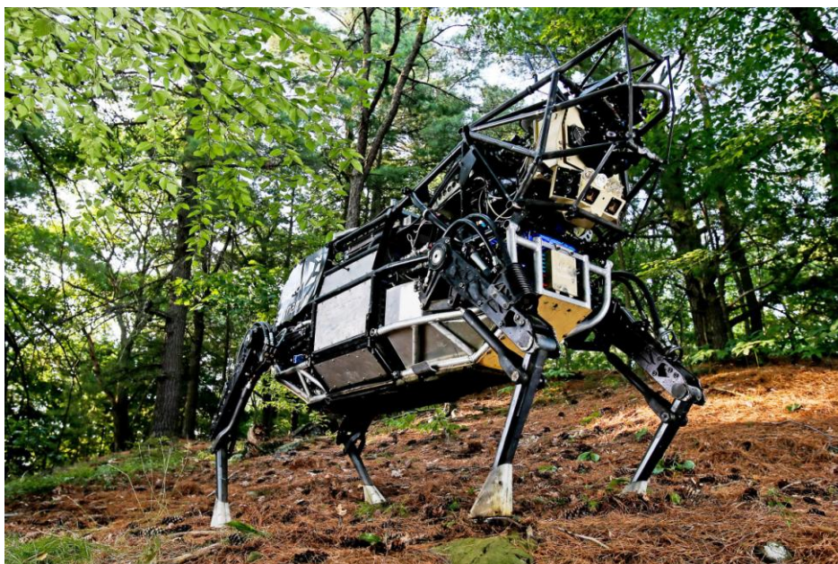
FIGURE H-3 LS3, Legged Squad Support System. SOURCE: Re-printed courtesy of Boston Dynamics.
