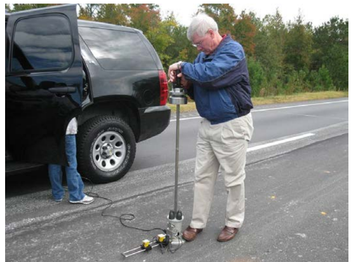
Figure 6.2. LWD testing on NCAT test track.
