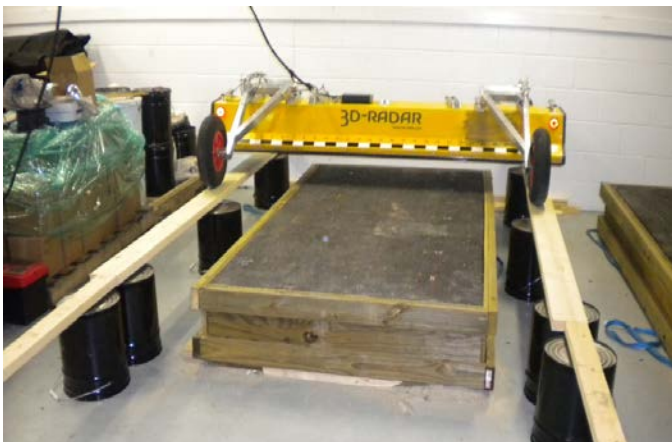
Figure 2.3. 3d-Radar equipment setup for laboratory slabs.
