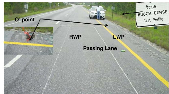
Figure 5.4. Approximate longitudinal zero point location for MIRA testing.
