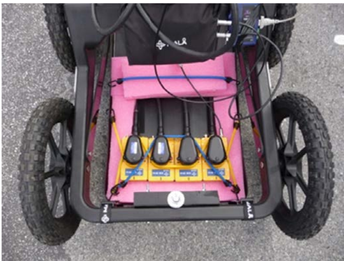
Figure 2.6. Testing of MALA systems at the test track: (a) MIRA system and (b) 2.3-GHz antennae in a cart.
