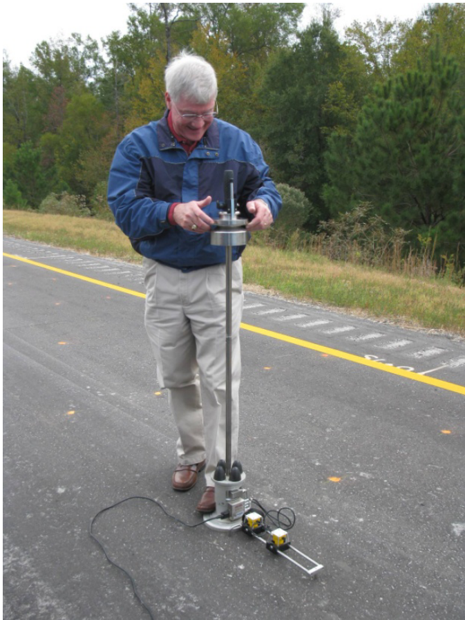
Figure 6.1. LWD testing on HMA pavement.
