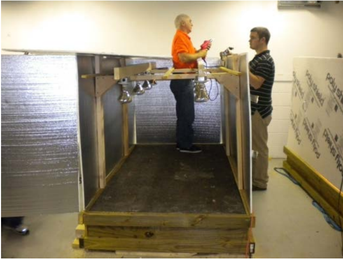
Figure 3.1. Heating of test slabs with heat lamps.
