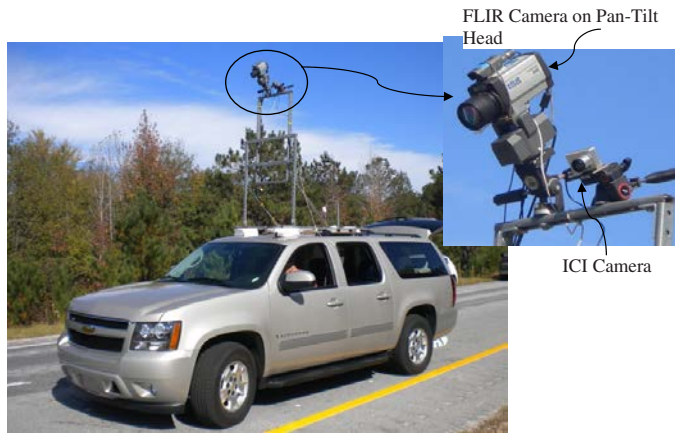
Figure 3.5. IR thermography setup for track testing.
