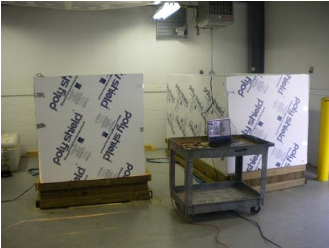
Figure 3.2. Test slab enclosure during heating process.
