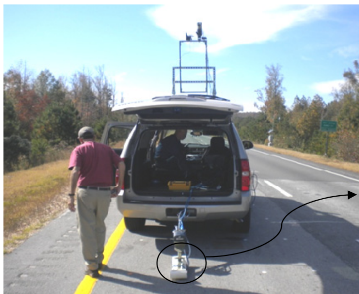
Figure 2.4. Deployment of the GSSI 2.6-GHz ground-coupled antenna pair.
