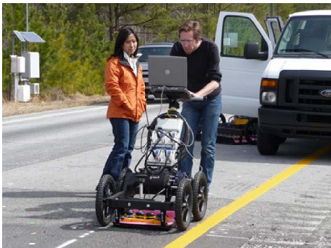
Figure 2.6. Testing of MALA systems at the test track: (a) MIRA system and (b) 2.3-GHz antennae in a cart.
