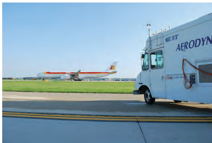
Figure 17. Mobile laboratory during PM tire and brake emissions measurements.
