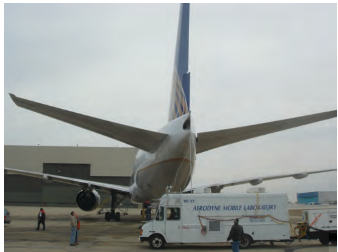
Figure 9. Measuring PM emissions from a GTCP 331-500 APU on a B777.
