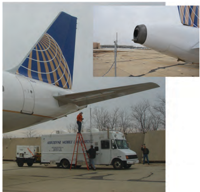
Figure 10. PM sampling probe behind an A320 aircraft with GTCP 36-300 APU.
