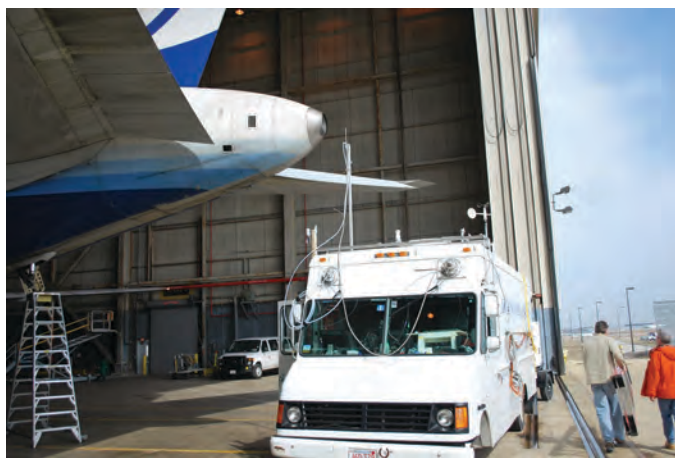
Figure 8. Aerodyne mobile laboratory positioned behind a B767 aircraft to measure PM emissions from the GTCP 331-200 APU.
