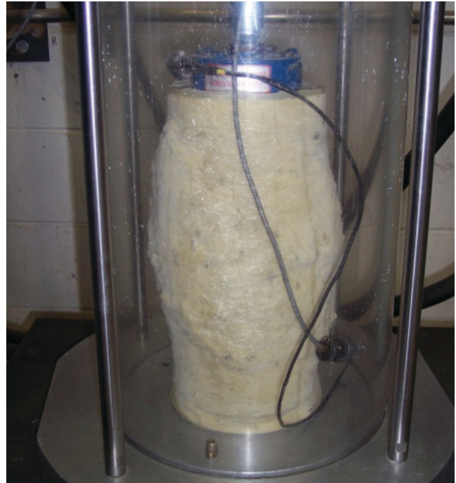
FIGURE 41 Deformed sample after completion of University of Illinois Rapid Shear Monotonic Triaxial Strength Test.
