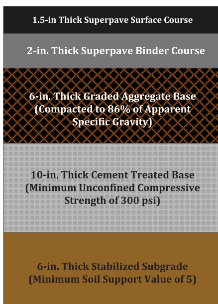
FIGURE 34 Schematic of inverted pavement section constructed in LaGrange Bypass Project, Troup County, Georgia.
