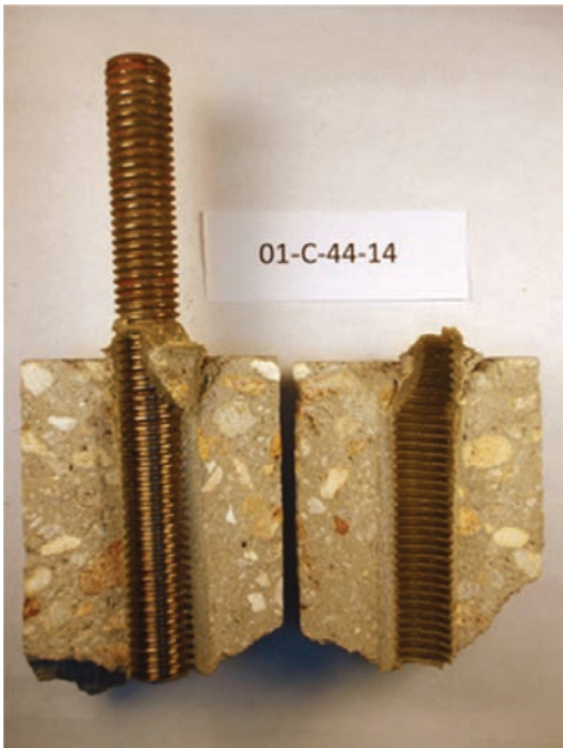
Figure 48. Typical terminated sample for adhesive C.
