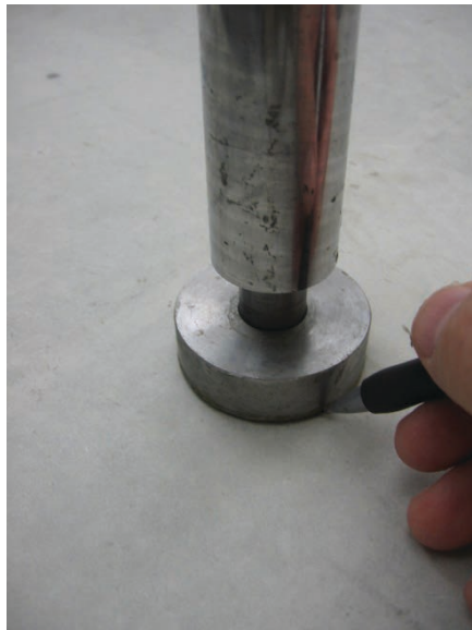
Figure 23: Centering tool inserted in hole.
