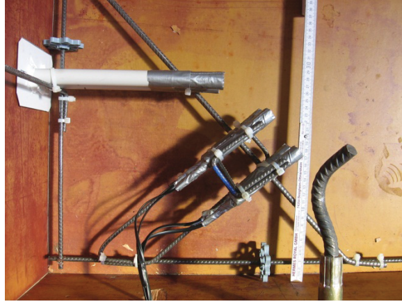
Figure 10: PVC pipes and Sensiron sensors placed in forms prior to casting.
