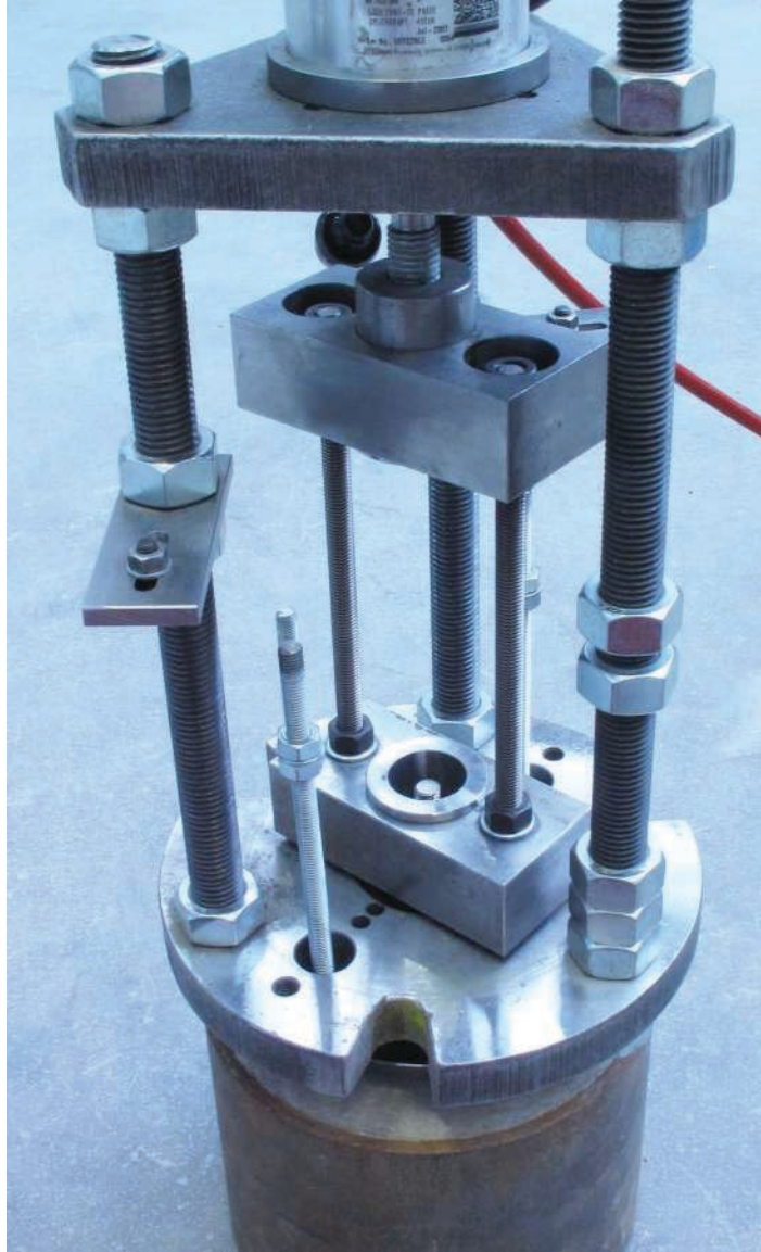
Figure 5: Coupler installed between loading rod and anchor.
