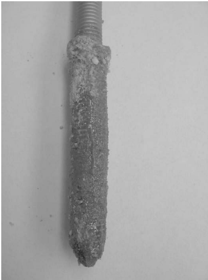
Figure 110. D21-C-ST-4 showing failure surface of incompletely cured specimen.
