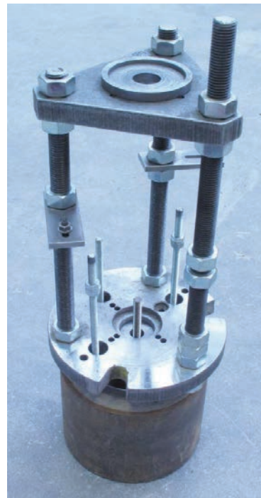
Figure 3: Tripod on top of the test specimens.
