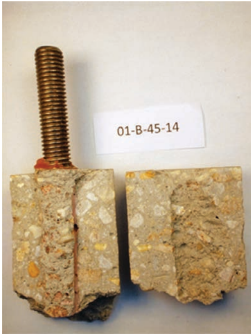
Figure 47. Typical terminated sample for adhesive B.
