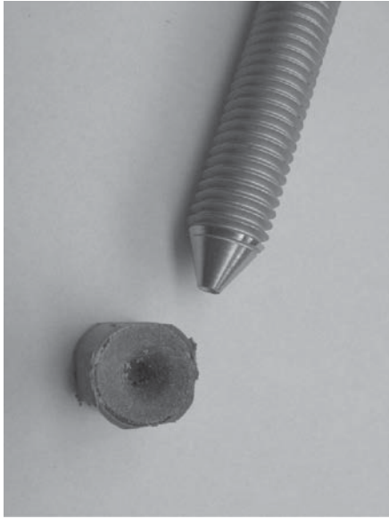
Figure 24: Centering guide with anchor.
