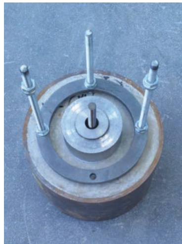
Figure 2: Transducer mount on top of the test specimen.
