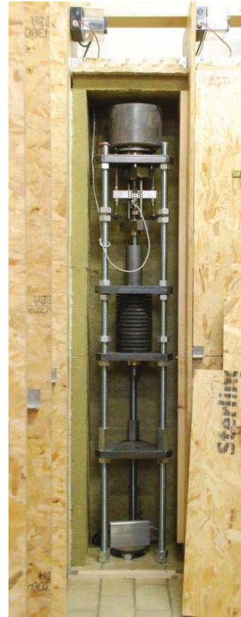
Figure 9: Small heating chamber (containing a single test rig).
