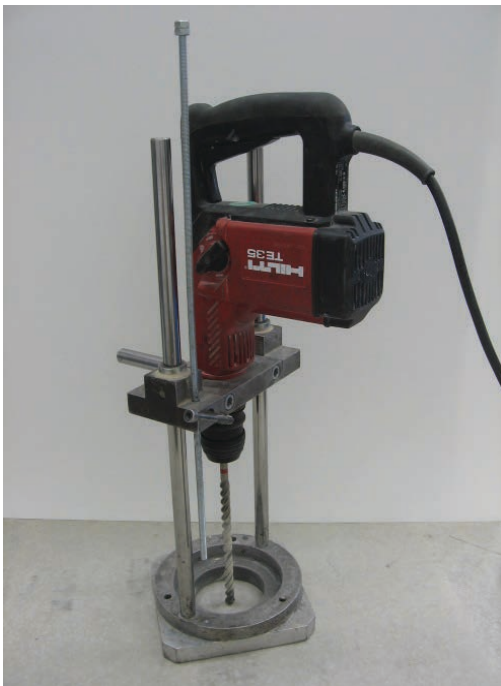
Figure 20: Drilling rig and hammer drill.
