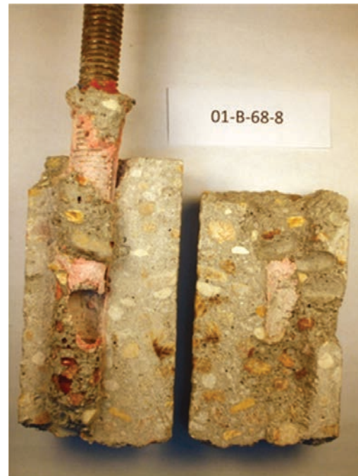
Figure 52. “Plug and reattachment” failure with concrete fracture.
