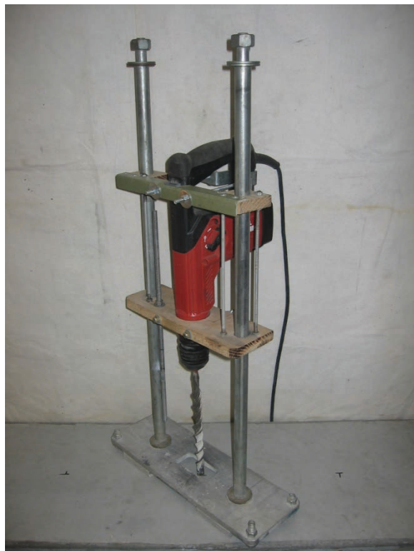
Figure 21: Drilling rig and hammer drill.
