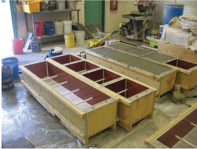
Figure 6: Concrete test specimens being cast.
