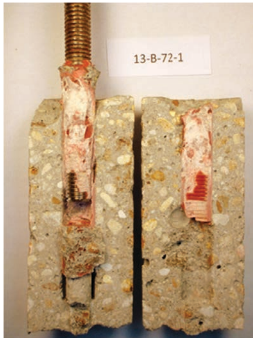
Figure 51. “Plug and reattachment” failure with thread separation.
