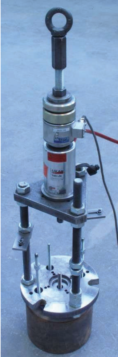
Figure 4: Hydraulic ram and load cell on top of the tripod.
