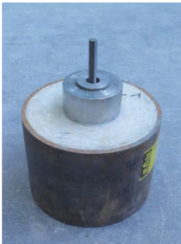
Figure 1: Test specimen with PTFE sheet and confining plate installed.
