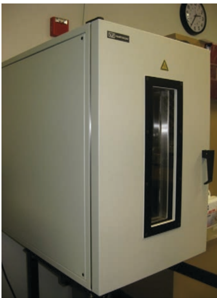
Figure 2: The oven, which pulls forward around the INSTRON, used to keep the samples at temperature.
