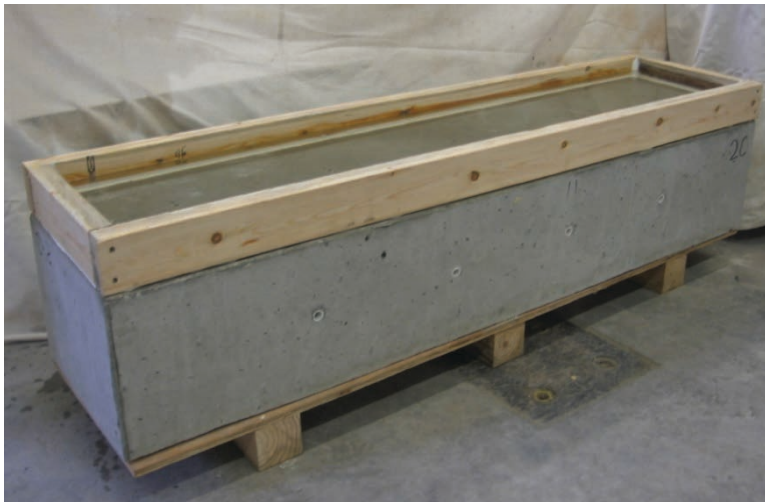
Figure 24: Water dam for test series 7 installation.
