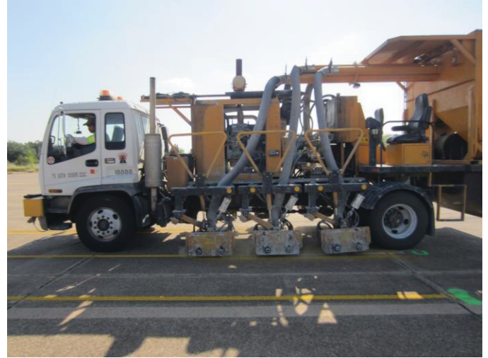
Figure 5. Full-size flailing drum-style removal truck.
