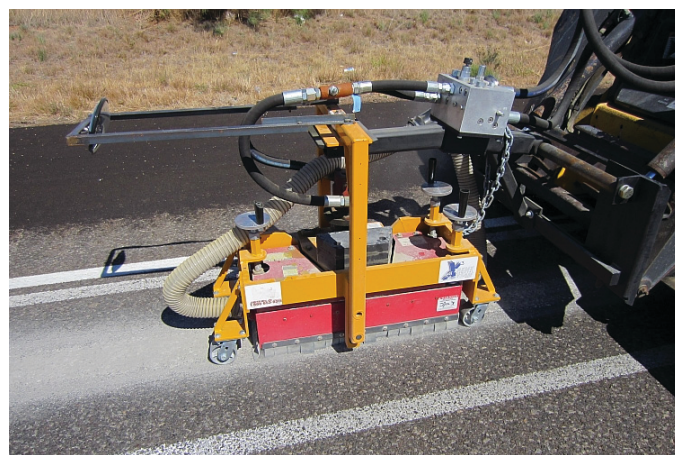
Figure 14. Orbital flailing on asphalt test deck.
