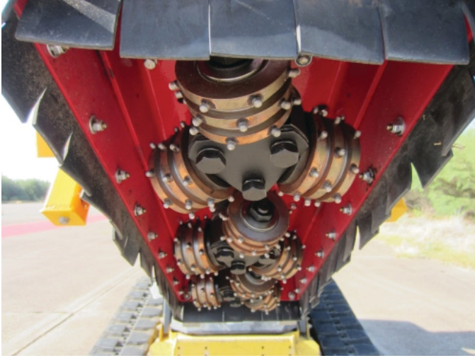
Figure 3. Orbital flailing style system mounted on track steer.
