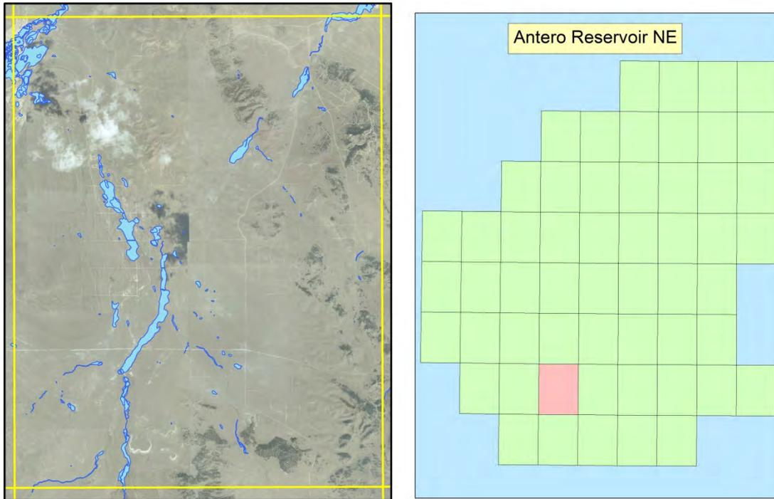
**Figure D.4.** Wetland polygons mapped within the Antero Reservoir NE quad shown over 2009 true-color aerial photography (left). Location of Antero Reservoir NE quad in relation to all quads in the study area (right).
