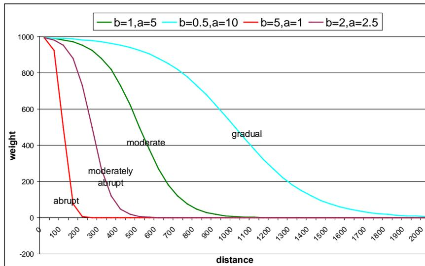
**Figure 1.23. As an example, for a total distance of 2,000 meters, different values of a and b produce the following curve types.**
