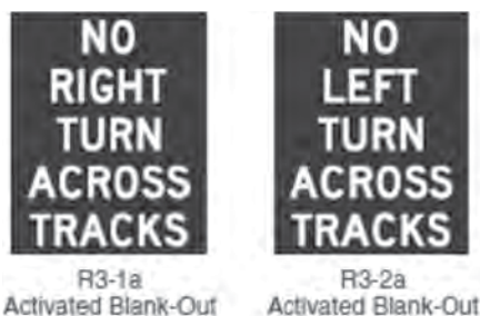
FIGURE 5 Dynamic turn restriction signs for rail crossings.
