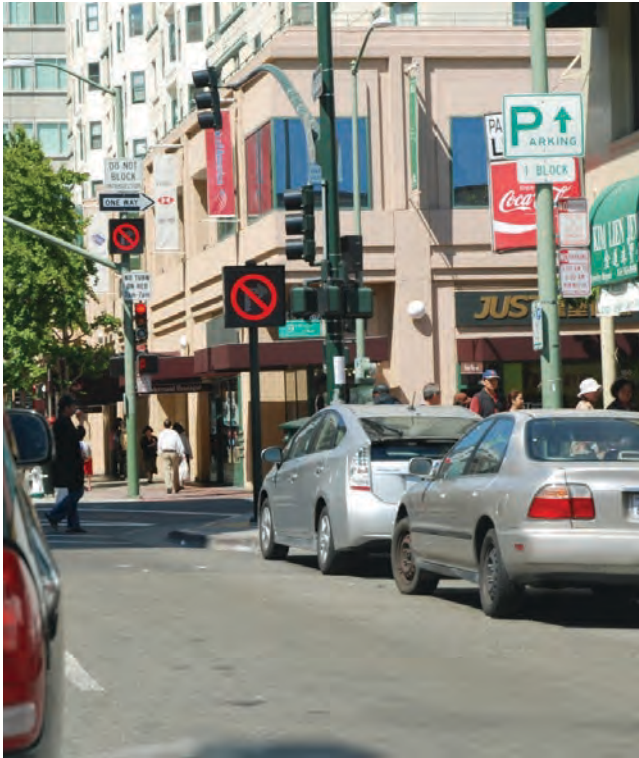
FIGURE 4 Example of a dynamic right-turn-on-red restriction, at intersection of Ninth and Franklin Street, Oakland, California (2012). Source: Kittelson & Associates.
