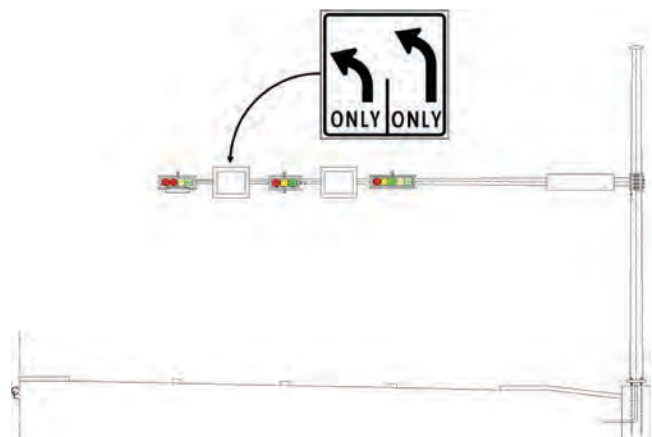
FIGURE 16 Planned dynamic turn lane installation—intersection of Louetta Road and Kuykendahl Road. Source: Andrew Mao, Harris County, Texas.
