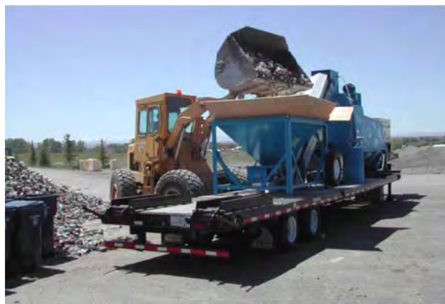
FIGURE 18 Portable glass crushing unit used for Montana pilot projects. http://www.astswmo.org/files/meetings/2006AnnualMeeting/Montana's%20Glass%20Aggregate%20compressed%20file.pdf .
