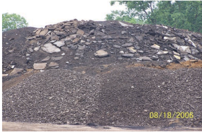
Figure 6. Multiple-source RAP pile with dirt contamination on the right side of the photo.
