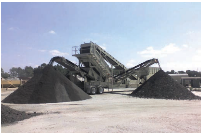
Figure 11. Portable RAP fractionation unit. This unit screens RAP into three sizes: +\frac{3}{4}'' on right, -\frac{3}{16}'' on left, and \frac{3}{4}'' \times \frac{3}{16}'' in back.
