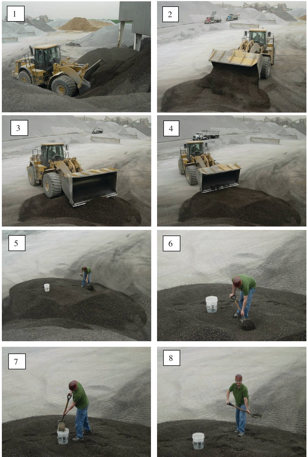
Figure 15. Steps for the best method to sample RAP.
