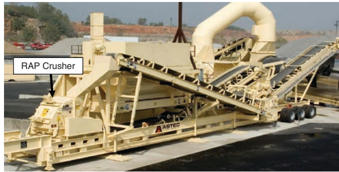
Figure 8. RAP processing unit with a screen before the crusher.
