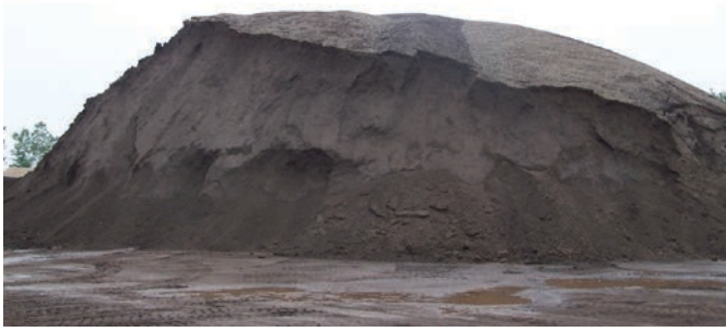
Figure 14. Processed RAP with a uniform appearance.
