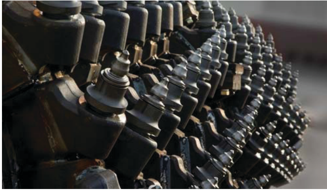
Figure 4. Micro-milling drums have three times the number of teeth as a normal milling drum.
