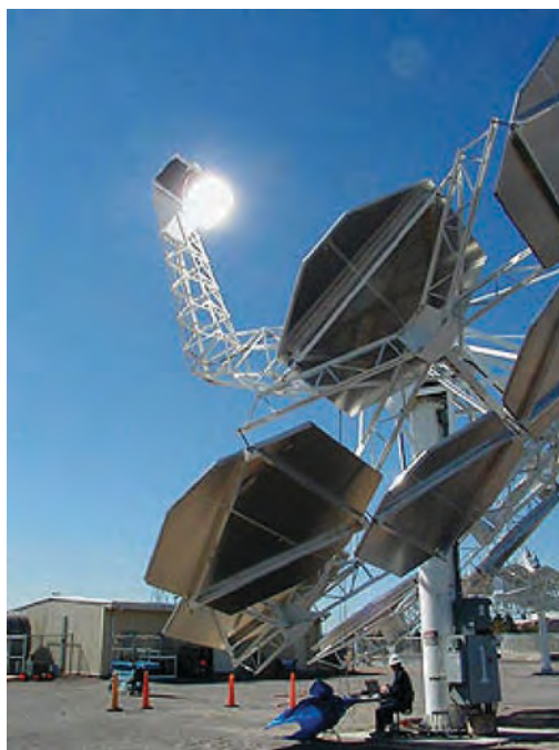
Figure 12-2. 25-kW solar dish Stirling engine system.
