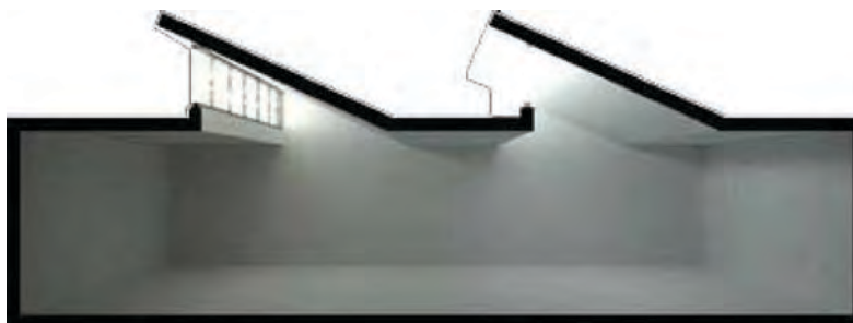
Figure 7-2. Sawtooth roof monitor providing top lighting, EcoTect model.
