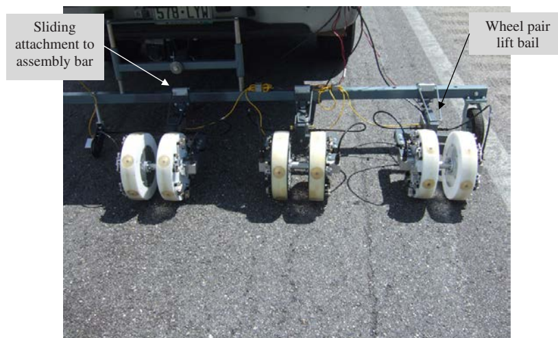
Figure 2.6. Current IE/SASW scanning system, showing the sliding connection system and lift bails.
