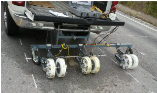
Figure 2.15. Test setup for IE and SASW at NCAT test track.
