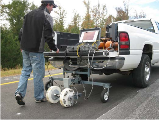
Figure 2.2. Scanning IE/SASW testing performed during Phase 1 on the NCAT test track.
