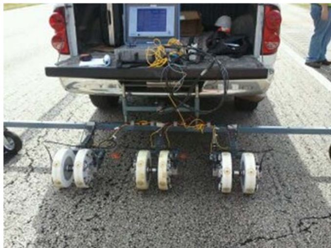
Figure 2.28. Test setup for Florida test site with six transducer wheels.
