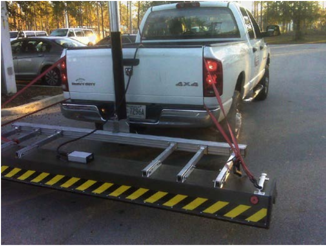
Figure 1.1. Antenna array and tower mount in position for data collection.
