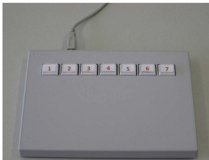
Figure 7.1. Button box used for driver survey response entry.
