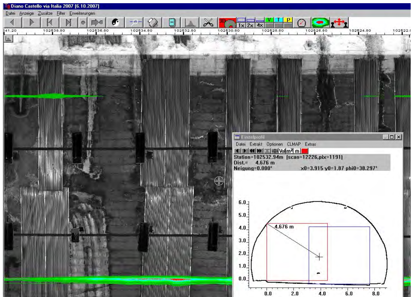
Figure I.4. Structural gauge investigation in motorway tunnel. Red spots indicate obstructions to given clearance profile. Users can determine cut volume and affected area on screen.
