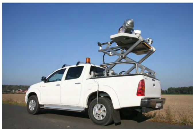
Figure J.6. Category A laser scanner survey system used in this research.
