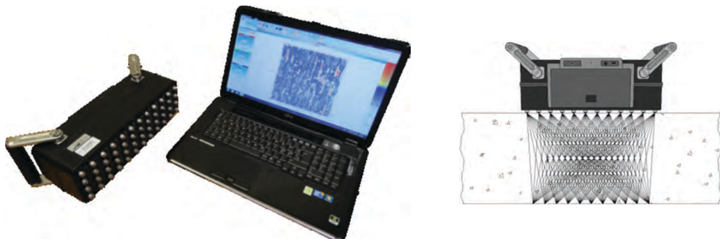
Figure 2.14. A1040 MIRA system (left) and transmission/reception of acoustic waves and corresponding echo intensity (right).
