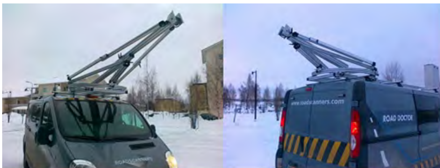
Figure J.17. New Roadscanners van roof-mounted rack system for laser scanner and thermal camera data collection.
