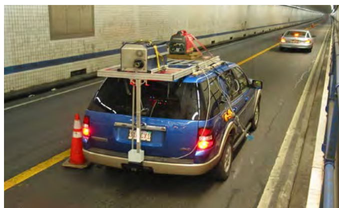
Figure I.7. Inspection vehicle in Chesapeake Tunnel.
