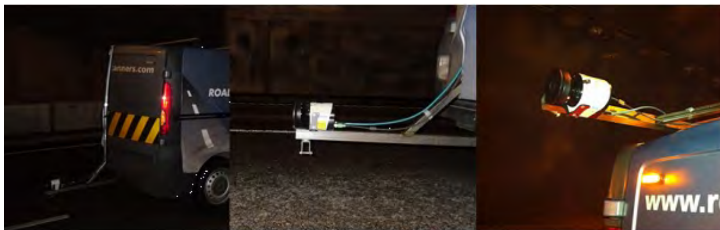
Figure J.7. Category B laser scanner mounting systems used in this research.
