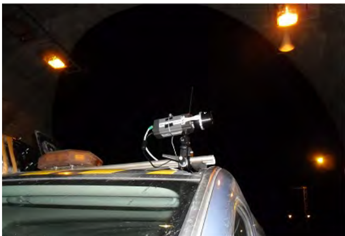
Figure J.4. Thermal camera installed on van roof in first measurement.
