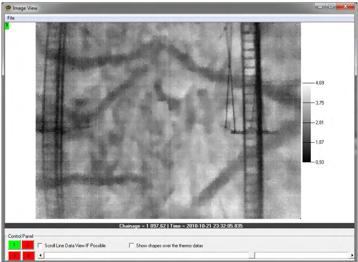
Figure J.22. Thermal video view in Road Doctor software display using example from Vuosaari Tunnel roof.
