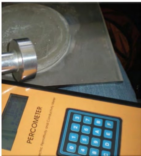
Figure S.4. Determination of percometer penetration depth with cement paste cast on stainless steel at different thicknesses. Probe of percometer uses a frequency of 40 MHz to 50 MHz.
