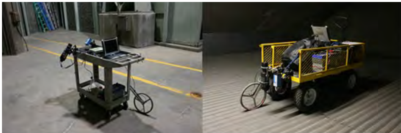
Figure J.16. Thermal video collection carts used in tunnel air duct measurements in the United States.
