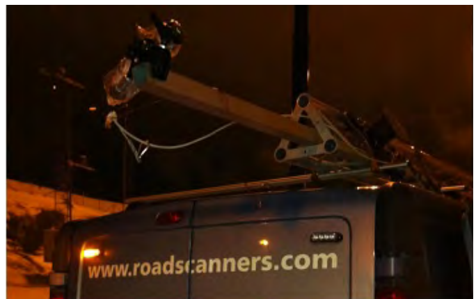
Figure J.5. Thermal camera installed on end of beam behind van.
