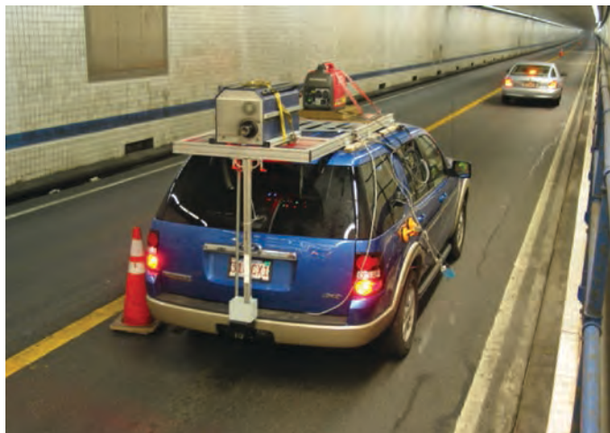
Figure 2.22. SPACETEC scanner in the Chesapeake Channel Tunnel.
