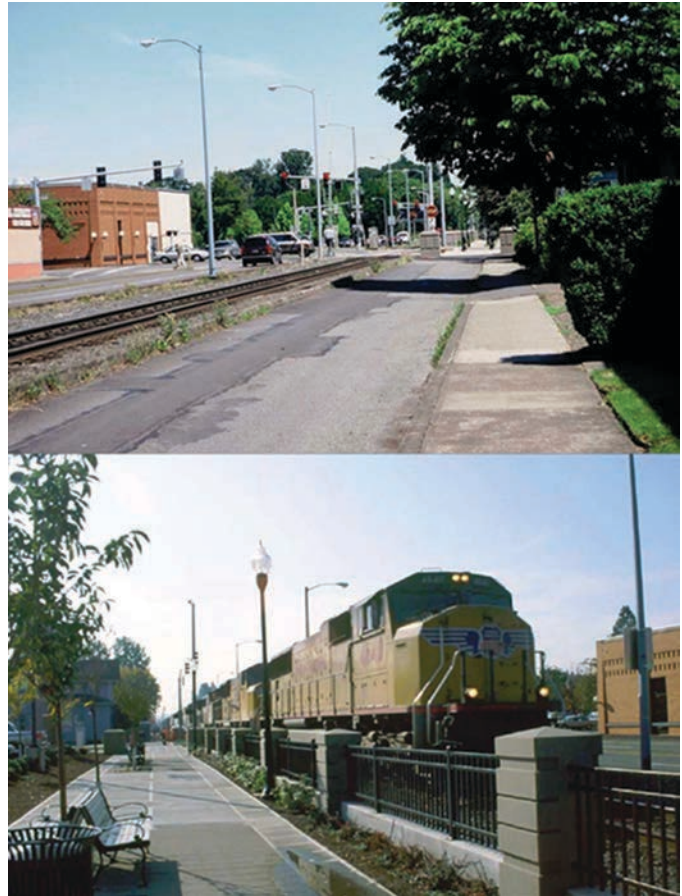
Figure 2.9. Barriers for pedestrian protection: before (top) and after (bottom).
