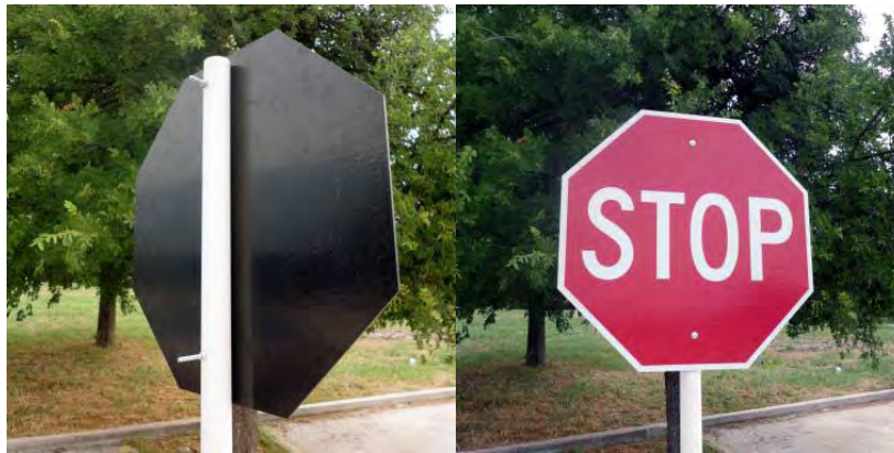
FIGURE 4 Stop sign manufactured with recycled ABS plastic.
