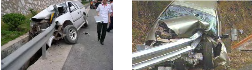
FIGURE 2 Unacceptable fishtail terminal performance.
