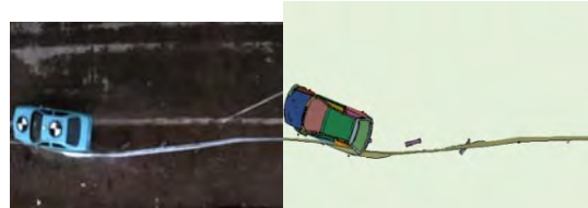
FIGURE 4 TB32 crash test and LS-DYNA simulation comparison for AG04-2.0 guardrail.
