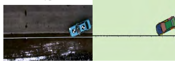
TB32 B-Type W-Beam Rail
