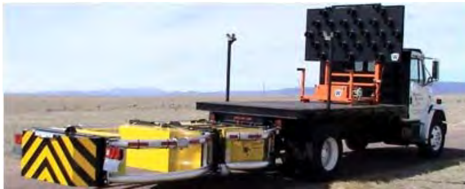
FIGURE 1 Example of a TMA.
