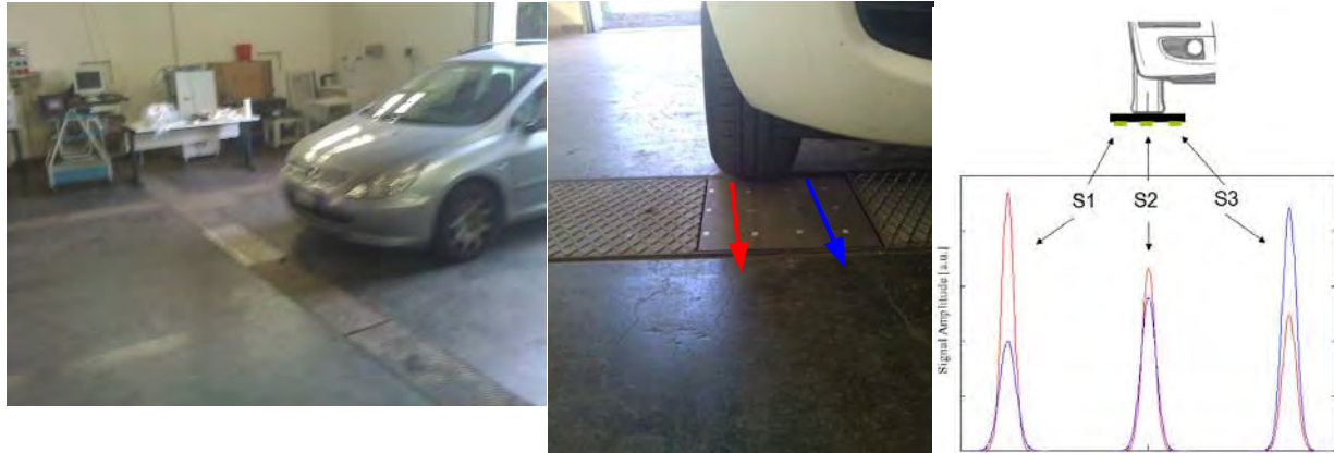
FIGURE 4 Experimental set-up for indoor WIM test at slow speed. Drawing on right shows dependence of sensors on position of transiting load: signals in red (blue) refer to load transiting on Sensor S1 (Sensor S3).
