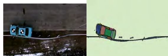
FIGURE 4 TB32 crash test and LS-DYNA simulation comparison for AG04-2.0 guardrail.
