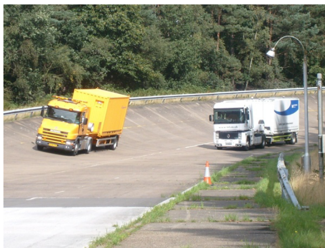
Figure 3.3. Two TSD devices at the Transport Research Laboratory (TRL) test track and a computer-generated schematic.
