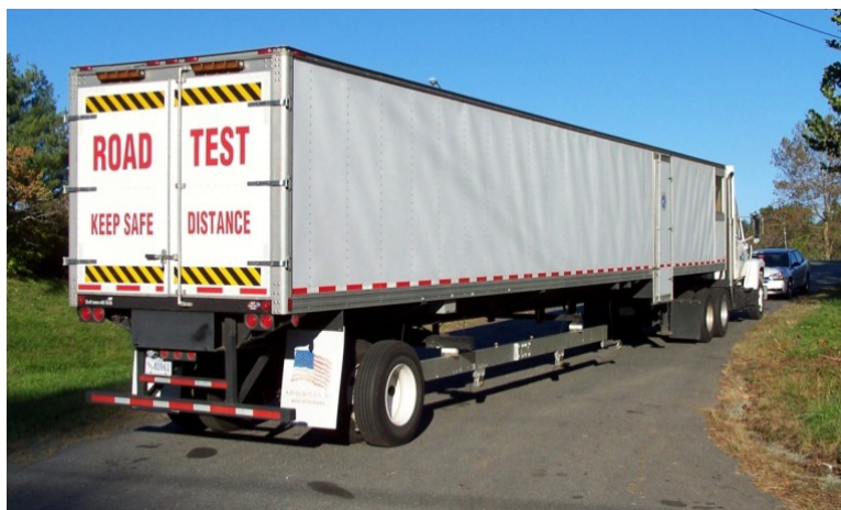
Figure 3.8. RWD during testing in Virginia and close-up of laser sensor placed between dual tires.
