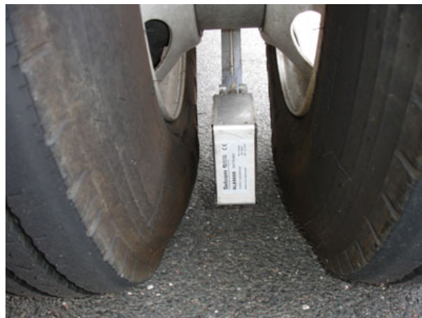
Figure 3.8. RWD during testing in Virginia and close-up of laser sensor placed between dual tires.
