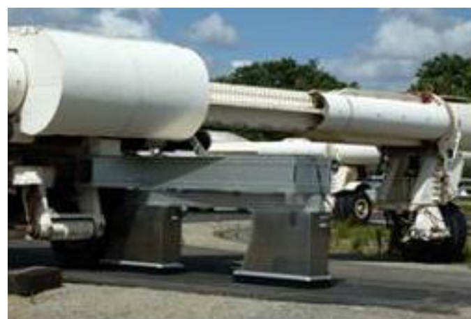
Figure 3.7. IDM prototype being tested at LCPC's pavement accelerated load facility.
