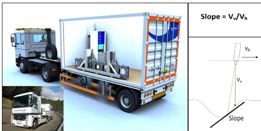
Figure 3.10. Computer render of the TSD, with the TSD in operation (inset).
