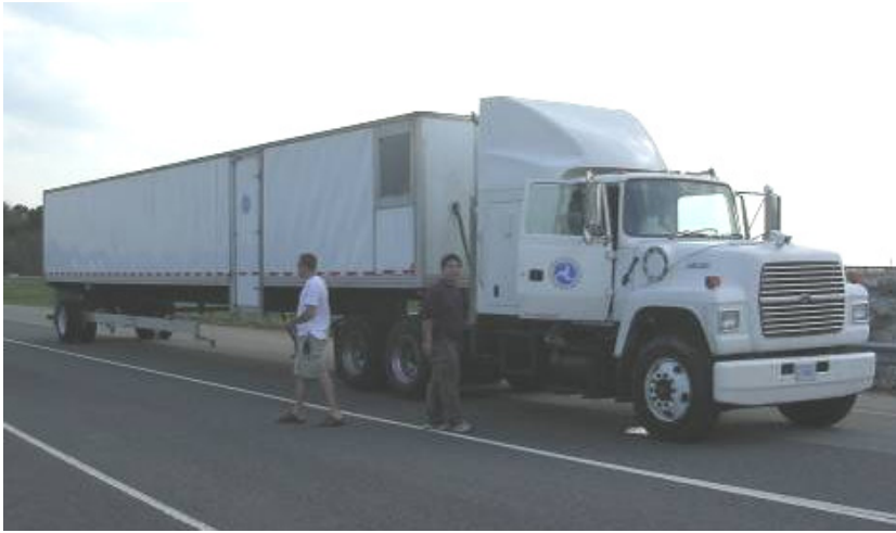
Figure 3.4. Rolling wheel deflectometer and its measurement principle.
