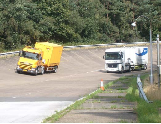
Figure 3.11. DRI device measuring side by side with the U.K. TSD at TRL in 2008.
