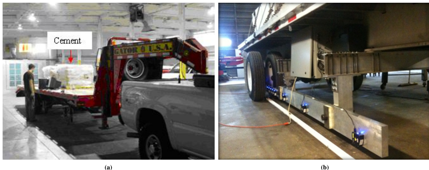
Figure 4.14. Eyztek Inc. lighter weight rolling weight deflectometer prototype: (a) frame view and (b) laser mounting beam.
