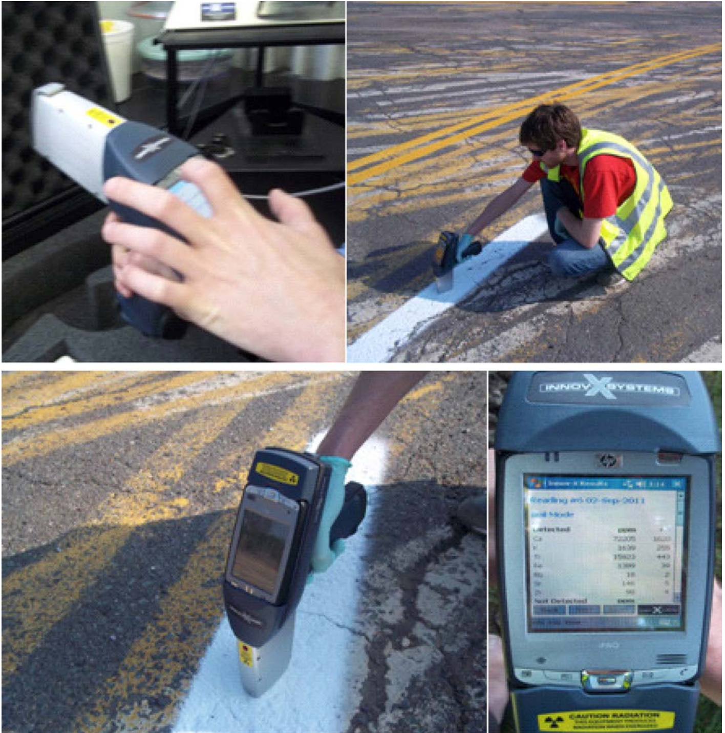
Figure Q.5. Device calibration (top left), white paint testing (top right), zoom on XRF instrument (bottom left), and image of XRF result screen (bottom right).
