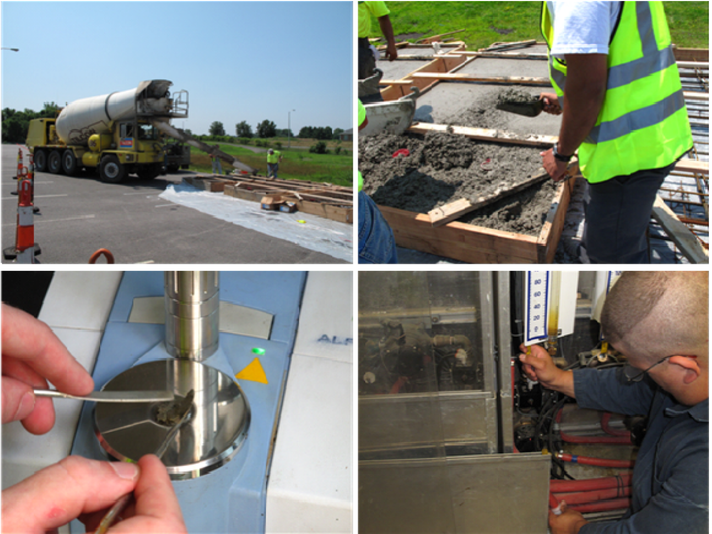
Figure Q.9. Pouring of PCC into a slab mold (top left), sampling PCC (top right), placing PCC sample onto ATR plate (bottom left), and sampling of chemical admixture (bottom right).
