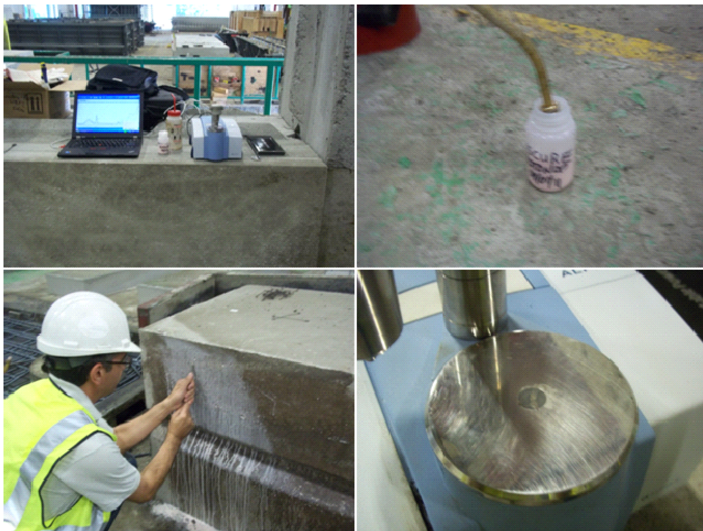
Figure Q.14. Equipment setup (top left), pure TAMMSCURE sampling (top right), surface sampling (bottom left), and sample on ATR plate (bottom right).
