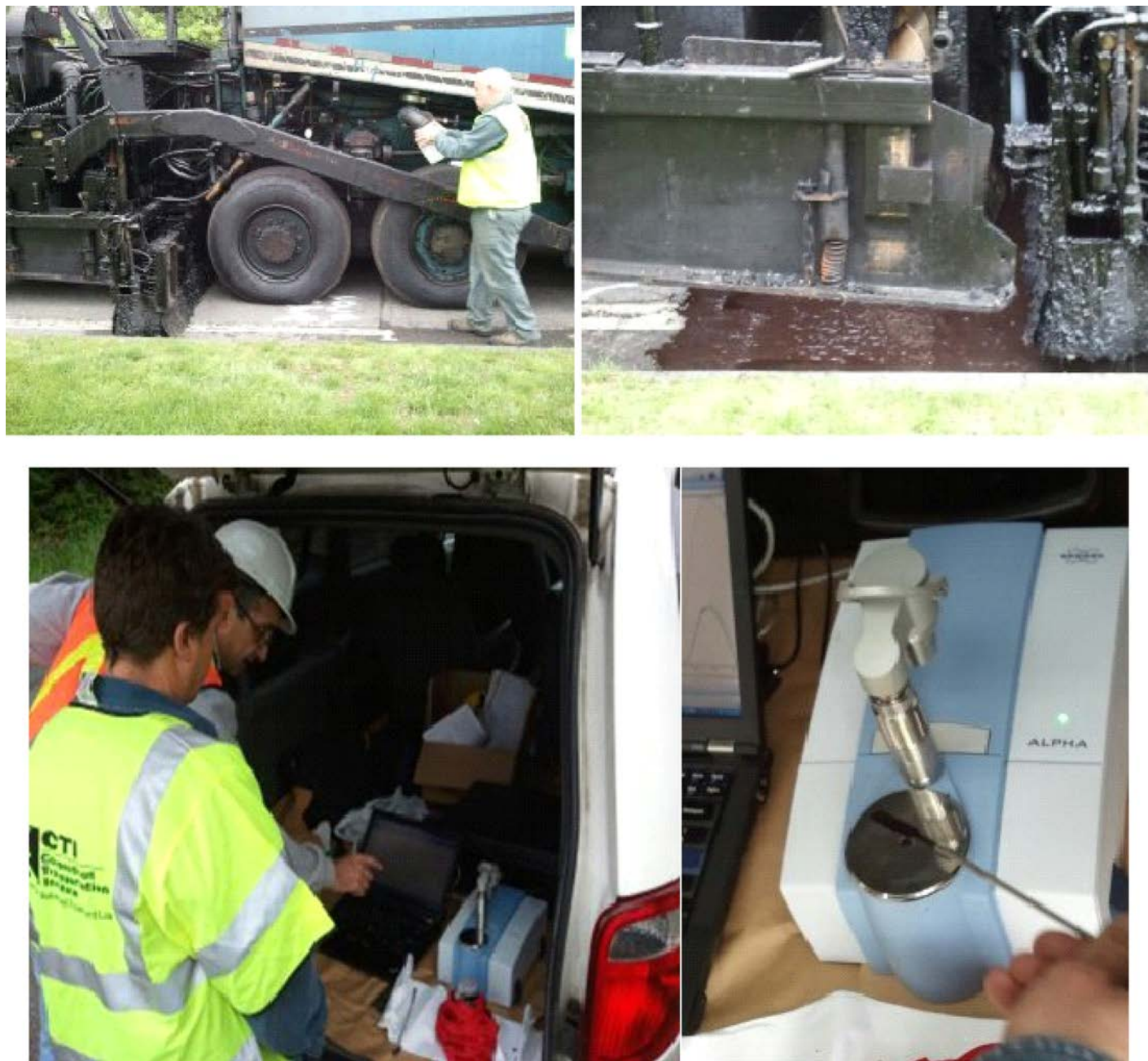
Figure Q.20. Sampling emulsion (top left), Novachip application (top right), ATR testing setup (bottom left), and sample placement (bottom right).
