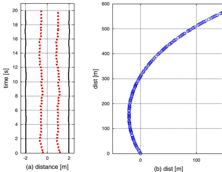
**Figure 7.11.** Vehicle path for Event 3. (a) The dotted lines represent the left and right edges of the vehicle with respect to the center of the lane markings (solid lines). (b) The XY position of the vehicle in space.
