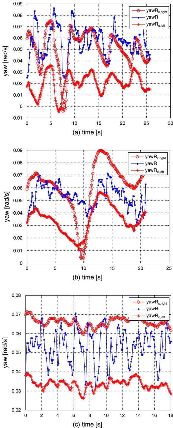
**Figure 7.13. Comparison between the critical yaw rate for left and right boundary conflicts and the actual yaw rate for (a) Event 1, riding the right boundary; (b) Event 2, single boundary crossing with correction; and (c) Event 3, good lane following.**
