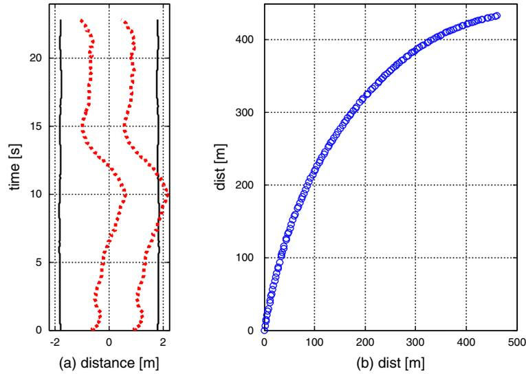
**Figure 7.7.** The vehicle path for Event 2. (a) The dotted lines represent the left and right edges of the vehicle with respect to the center of the lane markings (solid lines). (b) The XY trajectory of the vehicle.
