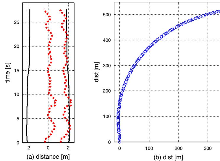
**Figure 7.3. The vehicle path for Event 1. (a) The dotted lines represent the left and right edges of the vehicle with respect to the center of the lane markings (solid lines). (b) The XY position of the vehicle in space.**
