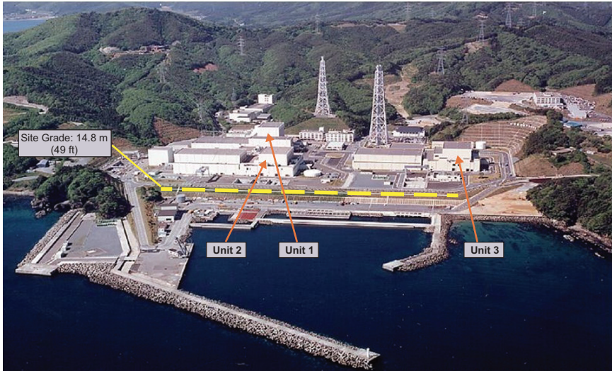
FIGURE 3.6 Oblique aerial photo of the Onagawa Nuclear Power Station prior to the March 11, 2011, Great East Japan Earthquake and tsunami. SOURCE: Courtesy of Tohoku Electric Power Company.
