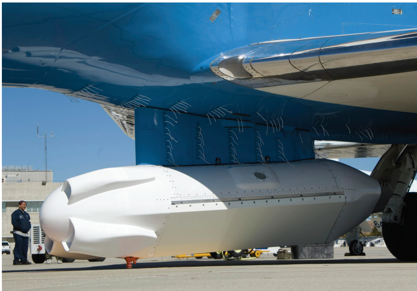
FIGURE 2.8 The AirMOSS sensor is located within the pod under the NASA Gulfstream III. SOURCE: Mahta Moghaddam, Principal Investigator, on behalf of AirMOSS EV-1 mission team.
