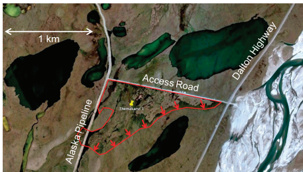
FIGURE 2.5 Thermokarst dynamics using InSAR. Anomaly in ALOS (Advanced Land Observing Satellite) subsidence trends near Deadhorse, Alaska (top). Google Earth image of thermokarst feature in Deadhorse, Alaska (bottom). Presented by Kevin Schaefer.
