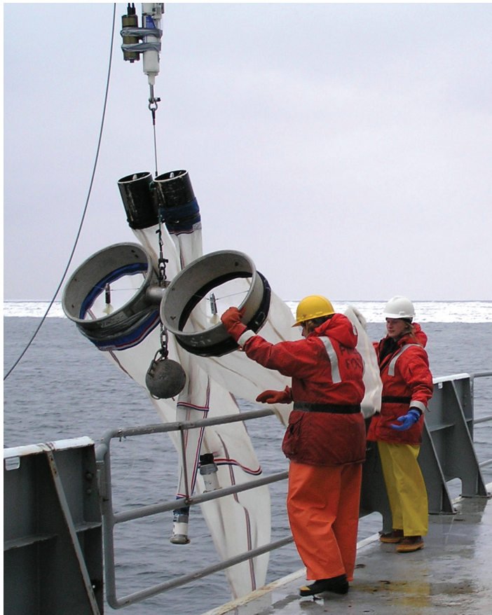
FIGURE 3.14 Researchers deploy a bongo net to sample zooplankton at the ice edge in the Bering Sea aboard the Research Vessel Thomas G. Thompson . SOURCE: NOAA.
