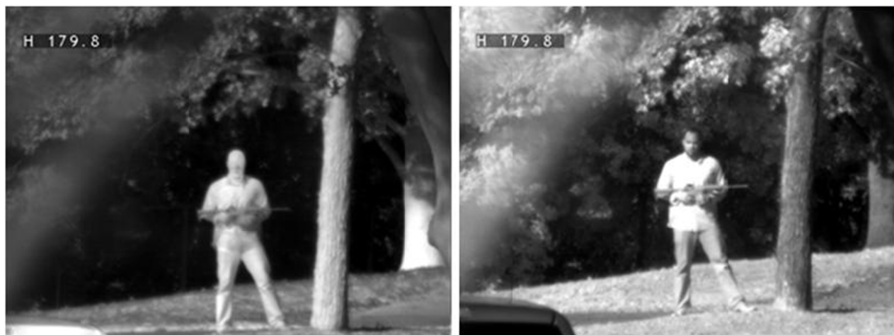
FIGURE 4-28 MWIR ( left ) and SWIR ( right ) imagery taken with a 640 \times 480 , 12 \mu\text{m} pixel camera operating at 150 K. SOURCE: DRS Technologies, Dallas, Texas.
