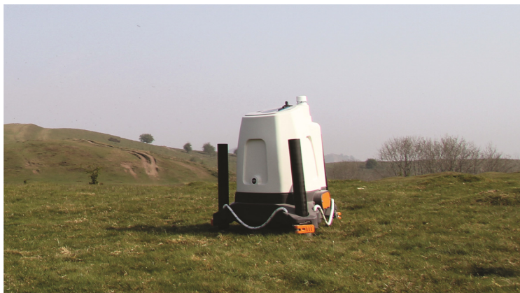
FIGURE 2-58 The ZephIR unit in the field. SOURCE: ZephIR 300 installed, image courtesy of ZephIRLidar.
