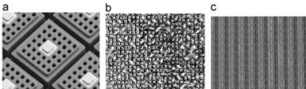
FIGURE 5-7 Grating light-coupling mechanisms used in QWIPs: (a) gratings with optical cavity, (b) random scattered reflector, and (c) corrugated quantum wells. SOURCE: A. Rogalski, 2012, “Progress in focal plane array technologies,” Progress in Quantum Electronics 36: 342, with permission from Elsevier.
