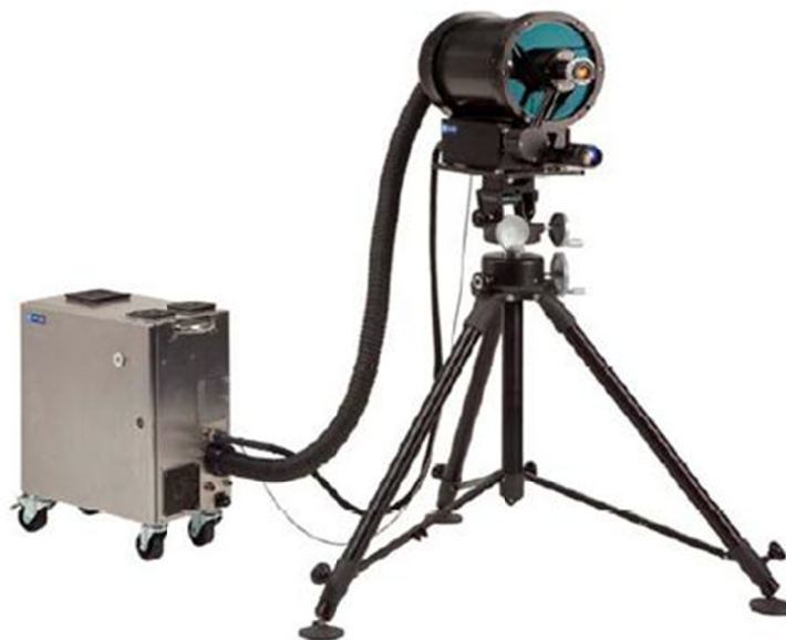
FIGURE 2-52 Photograph of Canadian-developed, bio-aerosol sensor (SR-Biospectra) designed for 100-m ranges. SOURCE: http://www.ino.ca/media/134174/srbiospectra.pdf .
