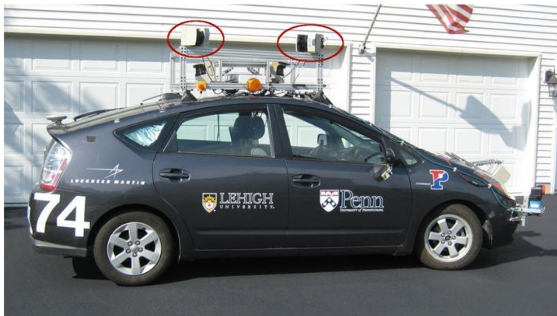
FIGURE 2-62 Ladders from SICK atop “Little Ben,” an experimental self-driving car developed for the 2007 DARPA Urban Challenge. Credited to Lehigh University.
