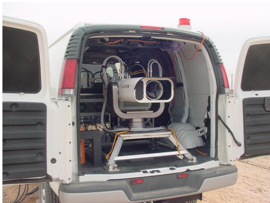
FIGURE 2-50 Photograph of the SNL-developed Ares aerosol and LIF lidar mounted in a van. SOURCE: http://www.sandia.gov/pcnsc/research/research-briefs/2004/Ares_Ultraviolet_Laser_Induced_Fluorescence_(UV_LIF)_Standoff_System_Development_and_Testing_by_R._L._Schmitt_et_al.pdf .
