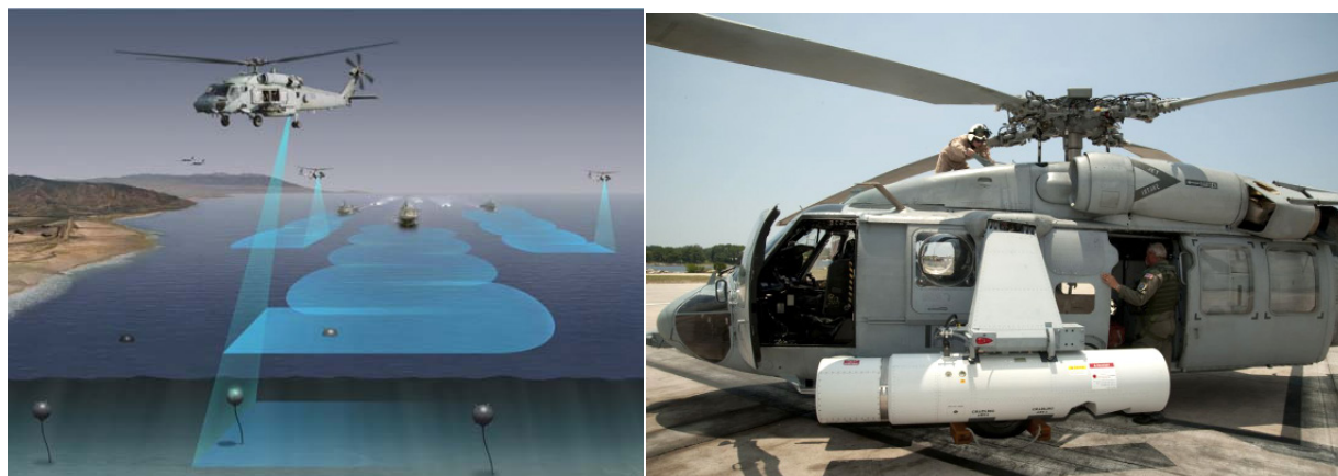
FIGURE 1-11 The Airborne Laser Mine Detection System (ALMDS). SOURCE: Photo credit: Northrop Grumman Corporation ( left ) and http://www.navy.mil/management/photodb/photos/100608-N-0001S-002.jpg ( right ).
