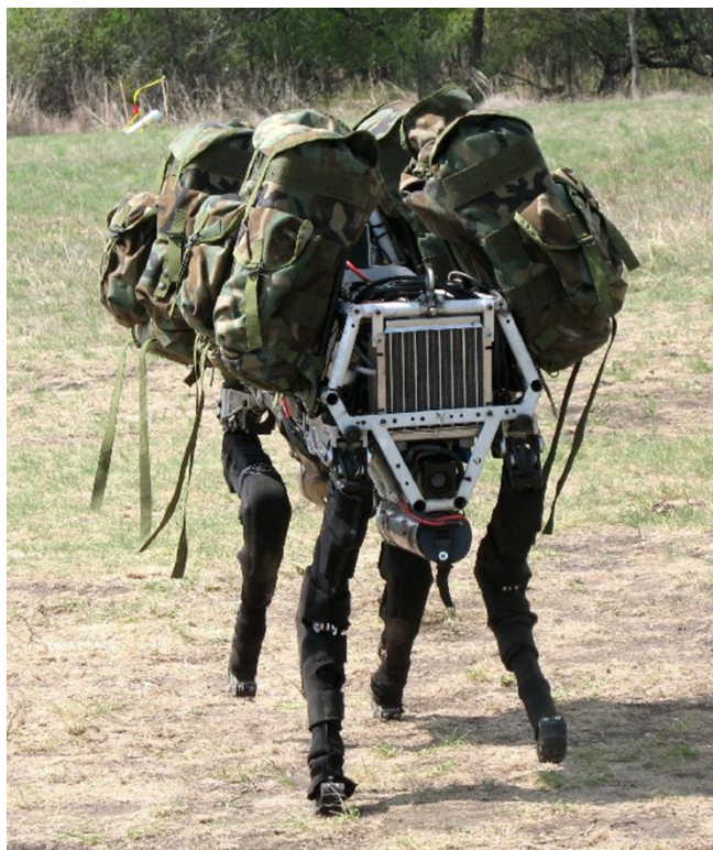
FIGURE 1-9 Boston Dynamics' BigDog quadruped robot. SOURCE: BigDog Robot image courtesy of Boston Dynamics.
