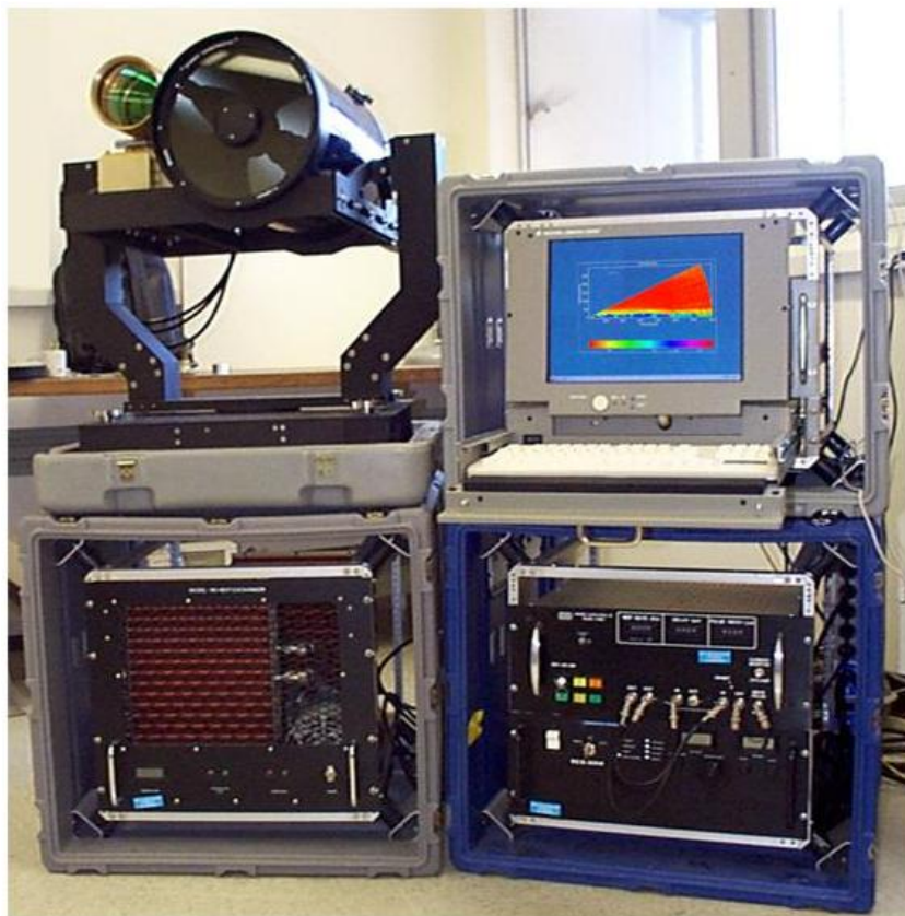
FIGURE 2-31 CLEAR aerosol lidar system developed for urban pollution measurements. SOURCE: Courtesy of Q-Peak, Inc.
