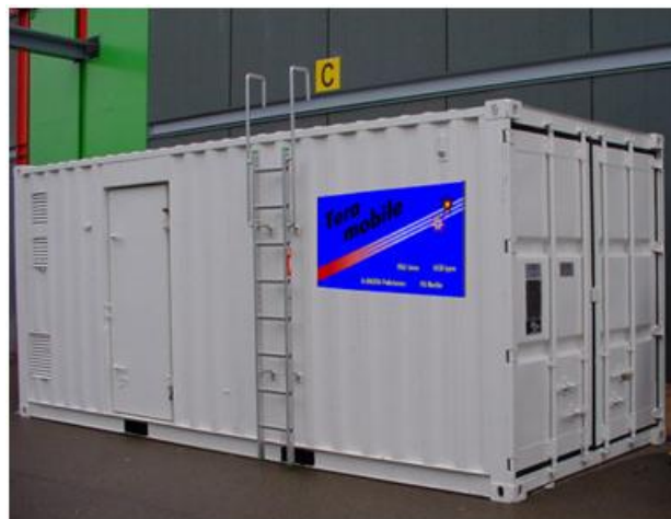
FIGURE 3-21 Plan for Teramobile lidar system ( left ) and photograph of system ( right ), built in a standard ISO 20 ft sea container. SOURCE: Copyright Teramobile. Used with permission.
