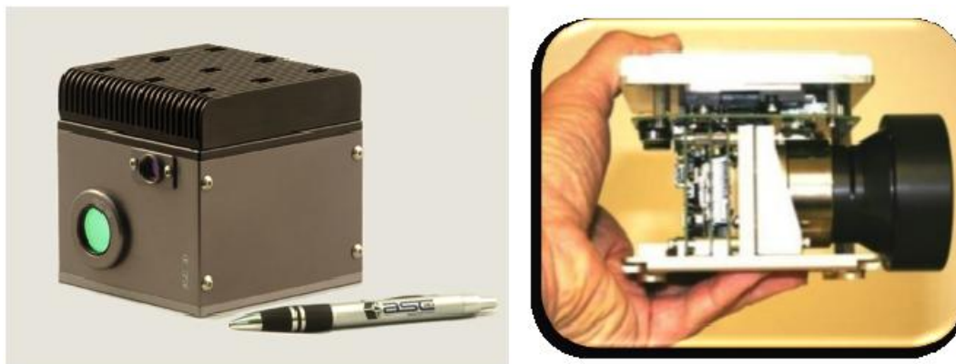
FIGURE 2-10 An early flash imager, ASC's 3-D FLC lidar. SOURCE: TigerEye 3D Flash LIDAR™ Camera (45° fixed lens); 2006 for robotics. Used by permission Advanced Scientific Concepts, Inc. (left). The TigerCub 3D camera captures 16,384 pixels with each laser pulse up to 30 frames per second. Used by permission Advanced Scientific Concepts, Inc. (right).
