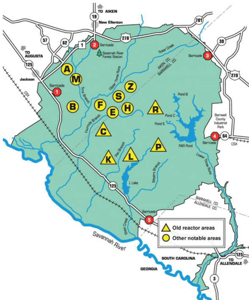
FIGURE 1-2 A map of the Savannah River Site. The triangles indicate locations of SRS's five production reactors (the C-, K-, L-, P-, and R-reactors). Circles indicate location of other major facilities including A: the Savannah River National Laboratory and the Savannah River Ecology Laboratory, M: fuel fabrication facilities, E: onsite disposal of low-level waste, H: H-canyon and the Tritium Extraction Facility (TEF), F: chemical processing (F-Canyon and FB Line) and tank farms, S: the Defense Waste Processing Facility (DWPF), and Z: the Saltstone facilities. SOURCE: http://www.srs.gov/general/tour/online.htm .
